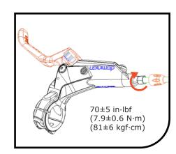
Bleed the brake (see bleed instructions) and clean with isopropyl alcohol, then slide the nose cone down to cover the compression nut.
