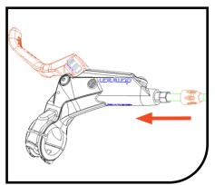
Using an 8mm crowfoot flare nut wrench torque the compression nut to 70±5 in·lbf (7.9±0.6 N·m, 81±6 kgf·cm).
