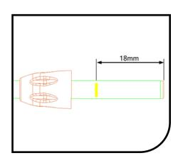
Push the hose completely into the master cylinder until it bottoms out. The 18mm line on the hose will sit flush with the end of the compression nut.
