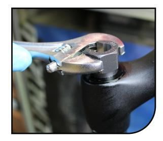
Remove compression damper assembly from the stanchion.
