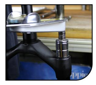
Attach a shock pump and inflate air leg 11 to 60PSI. This will aid in installing the casting later.
