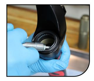
Fill the air chamber with air (60PSI). This will extend the air spring assembly and make casting installation easier.
