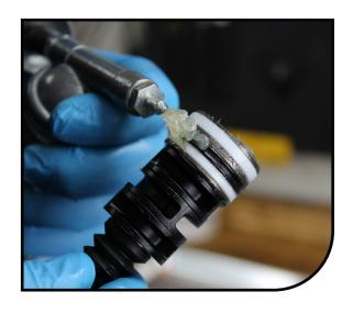
Add 8cc's of Slickoleum  $^{\mbox{\scriptsize TM}}$  grease to the top of the air piston.
