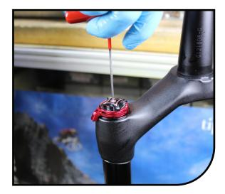
Clean fork and use a shock pump to set to desired pressure. Lightly pull the casing away from the CSA as you add air. Pressure chart below for reference.
