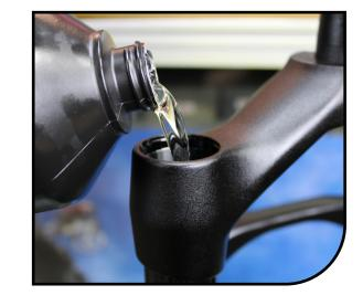
Place a lint-free towel over the opening in the damper leg and compress the fork 10-15 times.
