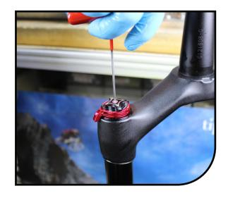
With a 13mm socket, unthread the exposed nut and remove the red low speed adjustment knob.
