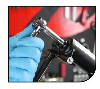
Insert an 8mm Hex wrench into the end of the rebound damper rod and turn the rod **clockwise** until it is disengaged from the casting and can be pushed into the casting.
