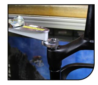
Secure red high speed knob adjustment knob with the 13mm nut using a socket, tighten down hand tight.
