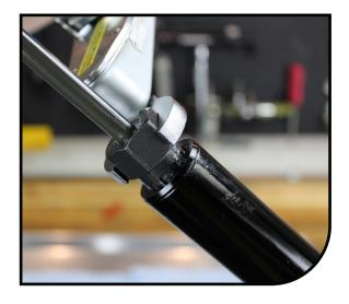
Install air cap onto stanchion. Tighten to 60-80 in lb [6.8-9.0 N m].
