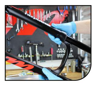
Insert 15cc's (15ml) of semi-bath into each casting leg. Once the semi-bath is in the legs slide the casting the rest of the way onto the stanchion assembly.
