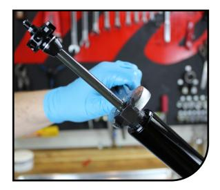
Remove air spring assembly from the stanchion. Clean spring and rod assembly with Isopropyl alcohol.
