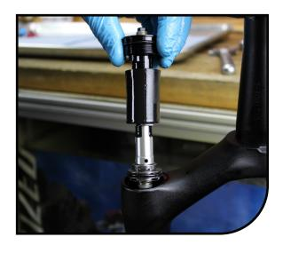
If installing an ABS+ damper use a 1" socket or crow's foot, the Manitou Cassette tool and a torque 60-80 in lb [6.8–9.0 N m].
