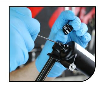
Remove IVA using a 24mm socket.
