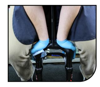
Pour additional fork oil into the damper leg until the oil height (space from the top of the damper leg to the top of the oil) is set at the proper level. See following page for the correct oil height depending on compression damper type and fork travel. An oil height setting tool used for motorcycle forks similar to the one pictured makes this job easier.
