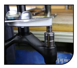
12 Attach a shock pump and inflate air leg to 60PSI. This will aid in installing the casting later.
