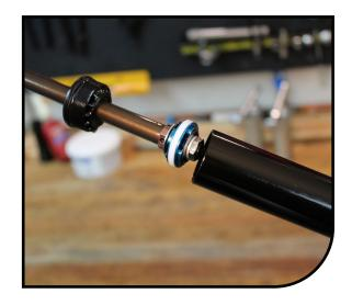
Install rebound damper into stanchion. Using the Mattoc cassette tool, a crow's foot and torque wrench, tighten the rebound damper assembly end cap to 80-100 in lb [9.0-11.3 N m].
