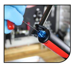
2 Insert an 8mm Hex wrench into the end of the rebound damper rod and turn the rod **clockwise** until it is disengaged from the casting and can be pushed into the casting.
