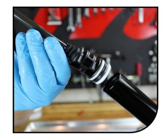
Once the air spring assembly is removed clean the inside of the stanchion with isopropyl alcohol and a lint free towel (Be careful to not scratch the inner surface of the stanchion). Inspect the inside and outside of the stanchion for scratches or other damage.
