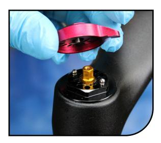
Unthread ABS+ compression damper assembly from the stanchion using a 24mm socket and ratchet.
