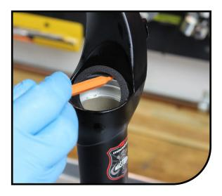
Remove springs from lip of dust seals. Clean seal area with Isopropyl alcohol. Using the Manitou 34mm Seal Press or large socket press in the dust seals. Reinstall springs onto seals.
