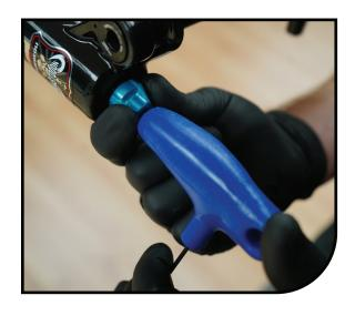
Hold lock-nut with 14mm end wrench for Pro & Expert, or a 19mm end wrench for Comp. Insert a 8mm Hex wrench into the end of the rebound rod and loosen clockwise until rebound rod disengages from the lock-nut.
