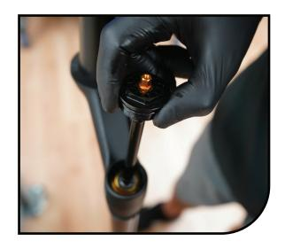
Tip out used damper oil from top of stanchion into drain pan. Cycle damper shaft serval times to cycle out old oil from damper.
