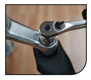
Pull IVA assembly straight out, Clean with isopropyl, Inspect seal for damage. If needed replace IVA piston seals.
