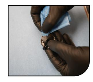
**Option:** ABS+ Install springs and ball bearings into ABS+ top cap. A small dab of grease on top of the spring can help hold the ball bearings in place.
