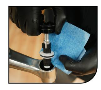
Invert the fork and use Manitou cassette tool with adjustable wrench to unthread the air spring assembly from the stanchion OR depress valve on end of comp-rod with 2mm hex and stroke rod to bottom. Slide standard cassette lock-ring tool over threaded adapter and unthread the air spring assembly from the stanchion.
