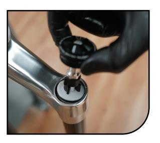
Install IVA cap into stanchion. Torque to 200-220 LB-in [22.6-25 Nm] using a 24mm socket.
