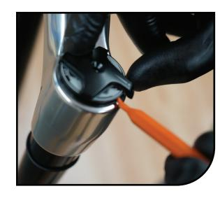
Remove the v-seal that was under the black VTT adjustment knob.
