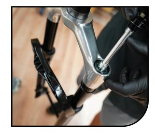
Clean the adjuster knobs with isopropyl and replace v-seal into damper top cap. Install the black VTT6 adjustment knob onto adjuster hex, being sure the knob can fully rotate without contacting the crown.
