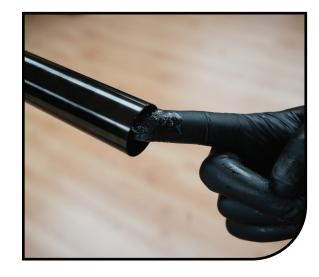
Install air spring assembly into stanchion. Using a 26mm crow's foot and Manitou cassette tool OR 1" Socket and Standard cassette tool torque to 40-45 LB-IN [4.5-5.1 Nm]. If rod is bottomed, attach shock pump to valve and draw the rod out until fully extended.
