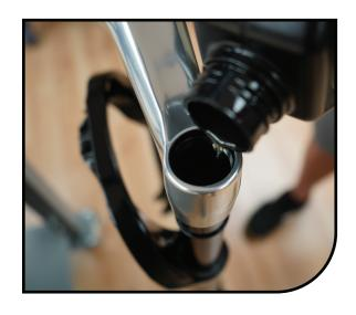
Install the axle into the fork without a hub or wheel. Cover the damper leg opening with a lint-free towel. Using a wood block or similar raised support underneath the axle, compress the fork 10-15 times.
