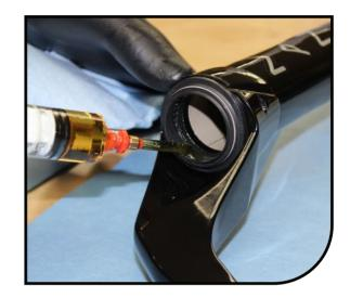
Make sure the spring shaft is fully extended and air chamber is filled with air (30 PSI).
