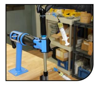
Fully extend damper shaft and add oil from bottom syringe until bladder is slightly expanded. Closing the bleed hose clamp on both syringes remove cartridge from vise. Lay cartridge flat on bench. Remove lower syringe and replace bleed screw. Some oil may discharge from bleed port when removing syring. Remove upper syringe and replace bleed screw.
