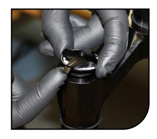
Remove the v-seal that was under the black VTT adjustment knob.
