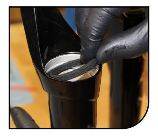
Remove springs from outer lip of new leg seals. Clean casting seal press area with Isopropyl alcohol.
