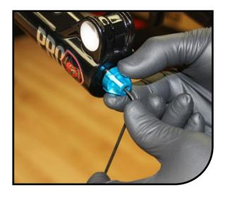
Thread the other lock-nut onto the spring shaft adapter. Holding the lock-nut with a 14mm Pro / Expert, 19mm Comp box wrench, use an 8mm socket tighten the compression rod adapter to 35–40 in-lb [3.95–4.5 Nm] by turning them **counter-clockwise.** Do not overtighten, doing so can damage the threads.
