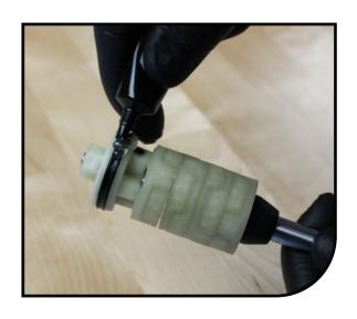
Add Slickoleum™ grease to the stanchion threads before inserting the air spring assembly. Spread grease across entire thread surface.
