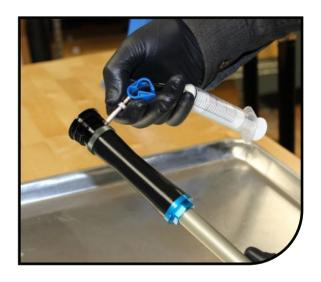
Holding the damper end-cap up-right in vise simultaneously compress the filled syringe and retract the empty syringe to remove air from the damper. Refill the syring as needed until oil is drawn into the upper syringe.
