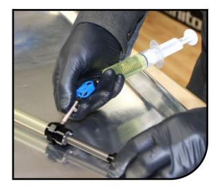
Attach the empty syringe M5x.8 adapter to top-cap bleed port. Remove bleed-screw from damper end-cap and attach the filled syringe M5x.8 adapter to end-cap bleed port.
