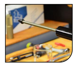
Fully extend the damper shaft.
