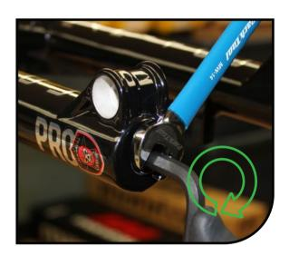
Unscrew air cap and attach shock pump. Depress pressure bleed button until pump reads "Zero".
