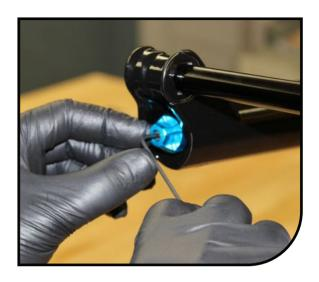
Thread the other lock-nut onto the spring shaft adapter. Holding the lock-nut with a 14mm box wrench, use an 8mm socket tighten the compression rod adapter to 35–40 in-lb [3.95–4.5 Nm] by turning them **counter-clockwise.** Do not overtighten, doing so can damage the threads.
