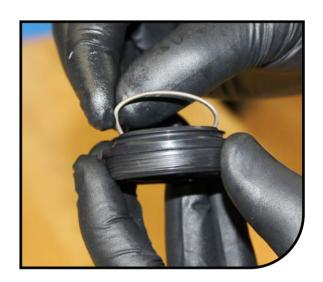
9 Using the Manitou 34/37mm Seal Press, press in the dust seals. Reinstall springs onto seals.
