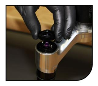
Remove detent balls and springs from the ABS+ top cap.
