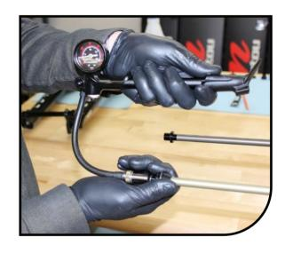
Fully extend the damper shaft.
