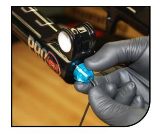
Hold lock-nut with 14mm end wrench for Pro & Expert, or a 19mm end wrench for Comp.
