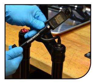
Attach a shock pump and inflate main air chamber to 60PSI. This will aid in installing the casting later.
