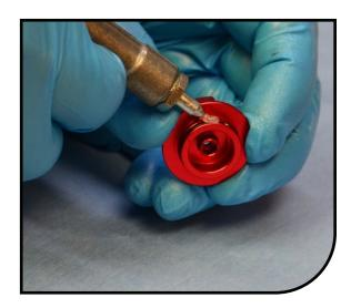
Lubricate o-ring seal on red "LO-SPEED" adjustment knob with Slickoleum<sup>™</sup> Grease an install onto adjuster hex. With a 2mm hex, thread on the screw and torque to 4-6 in-lb [0.5-0.7 Nm] Note: Be sure to hold the knob still while installing the screw. The damper adjuster may be damaged if the knob is over torqued.
