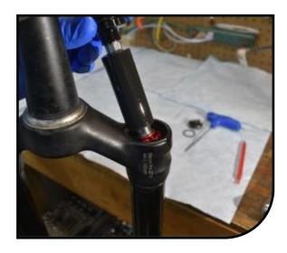
Clean the adjuster knobs with isopropyl and replace v-seal into damper top cap. Install the black VTT adjustment knob onto adjuster hex, being sure the knob can fully rotate without contacting the crown. With a 2mm hex, thread on the screw and torque to 4-6 in-lb [0.5-0.7 Nm] Note: Be sure to hold the knob still while installing the screw. The damper adjuster may be damaged if the knob is over torqued.
