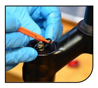
Use a standard cassette tool and 1" socket to unthread the damper top-cap from the stanchion.
