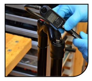
Mezzer Pro: Using a standard cassette tool and 1" socket loosen IRT cap until threads are free from leg. Mezzer Expert: Using a 24mm socket loosen IVA cap until threads are free from leg.
