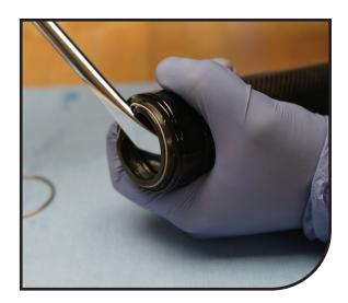
Remove the foam ring. Clean seal bore and bushing thouroughly.
