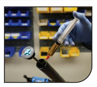
Fully extend the inner leg and tighten down the top cap using a 16 notch Bottom Bracket Tool to the proper torque of 6.8-9.0 N m (60-80 in lb). Reinstall the damping leg into the fork crowns on the bike.
