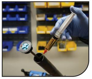
Replace the oil and dust seals on the outer leg following the directions on page 26-27. Inspect the inside of the outer leg, and be sure it is free from debris and contaminants. Coat the inside of the seal with Slickoleum grease. Slide the inner leg into the outer leg, and clamp the top of the outer leg in the bike stand.
