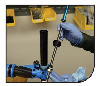
Carefully remove the A) glide ring (129-27922-L013), B) back up ring (129-31523-L338) and C) air piston quad seal (110-215). We recomend using a plastic pick to ensure the piston is not damage.
