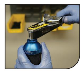
Release the air from the system. Remove the air caps from the top and bottom of the fork leg. Release the air pressure using a shock pump. Ensure all air is released by gently depressing the air shaft with a 3mm hex wrench.
