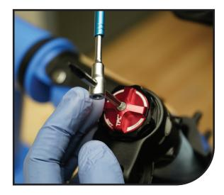
Remove O-ring and be sure you capture the 2 detent balls and springs under the knob.
