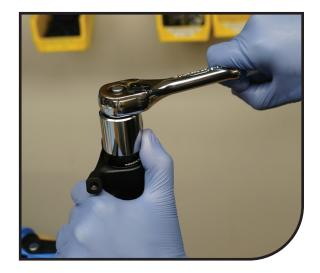
Inspect the inner leg, inside and out, clean it and be sure it is free from debris and contaminants. Lube the threads on bottom of the inner leg, lube the outer diameter of the IRT air piston and the exposed IRT shaft, and insert the assembly using a rotational motion.
