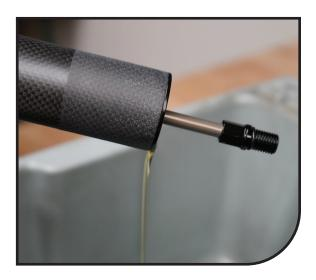
Pour the fluid out of the leg, and slide the inner leg out of the outer leg. Remove the outer leg from the stand and let it sit above a drainage pan.
