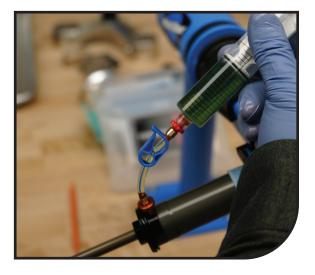
Return the cartridge to full extension, push oil from end cap to top cap.
