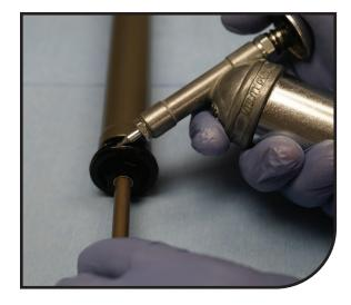
Install the assembly in the inner leg by sliding it into the bottom of the leg.
