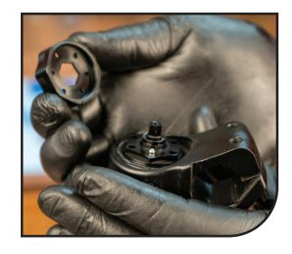
Loosen the damping leg top cap using a 16 notch
