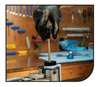
13 After you have properly set the oil height fully extend the inner leg and tighten down the top cap using a 16 notch Bottom Bracket Tool to the proper torque of 6.8-9.0 N m (60-80 in lb).
