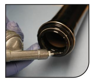
Install the top cap onto the end of the compression rod.
