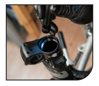
Apply a small amount of Slickoleum grease to the O-ring installed on the damper end cap. Install the assembly in the inner leg by sliding it into the bottom of the leg. Use a 26mm socket to tighten it into the leg. Tighten to 6.8-9 Nm (60-80 in lb).
