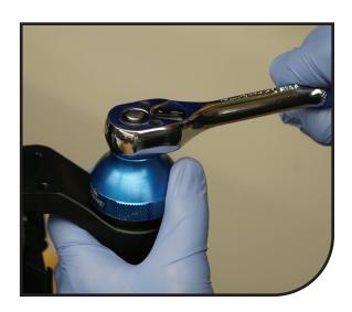
Loosen the pinch bolts on the lower crown, and remove the leg from the fork. Be sure not to misplace the frame bumper that will need to come off the fork leg.
