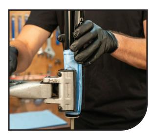
Remove the damping cartridge from the inner leg using a 26mm socket.
