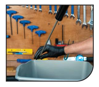
Wrap the inner leg in a rag and lightly clamp it into a bike stand with the rebound shaft pointing down towards the floor.
