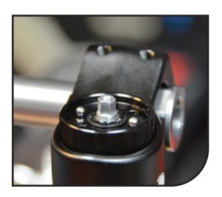
Place 0-ring # 100-024 around the TPC+ knob and apply a small amount of grease to it.
