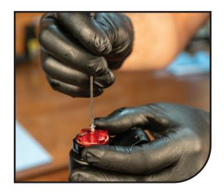
Remove 0-ring and be sure you capture the 2 detent balls and springs under the knob.
