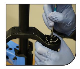
The air spring leg top cap needs to be loosened.
