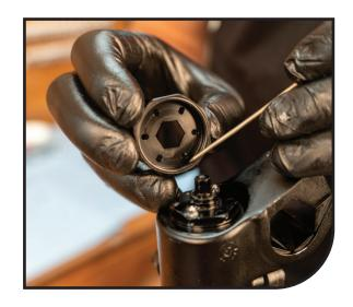
Insert the springs into opposite holes on the TPC+ adjuster knob and then place the detent balls in the corresponding holes of the high speed adjuster knob.
