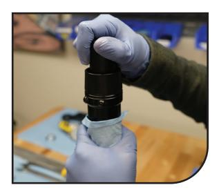
Install the wear ring back onto the outer leg.
