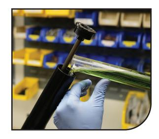
After damper is fully bled, fully extend the inner leg and tighten down the top cap using a 16 notch Bottom Bracket Tool to the proper torque of 6.8-9.0 N m (60-80 in lb).
