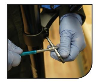
Lightly clamp the fork leg in a bike stand. Remove the top cap from the leg with a 16 notch Bottom Bracket Tool. Remove the top cap from the compression rod with a 14mm wrench on the top of the compression rod and a 16 notch Bottom Bracket Tool.
