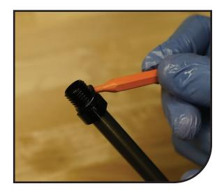
B. 0-ring # 100-026 - This is the 0-ring that is around the outside of the compression assembly top cap.
