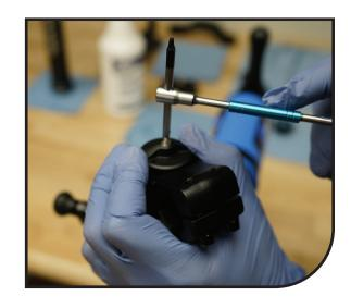
Be sure you capture the 2 detent balls and springs under the knob
