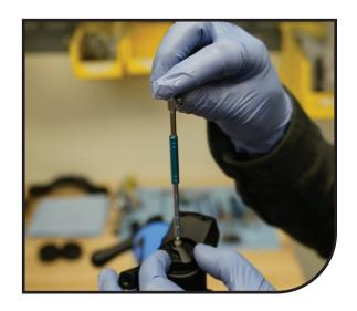
Using a 20mm socket loosen the bottom spring cap.
