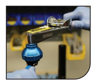
Install the rebound knob into the top cap by snapping it into place. Fully close the rebound by turning the knob clockwise.
