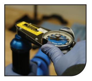
Using the sag guide tool to spread the crowns, slide the leg into the crown, align to proper wheel size and tighten crown bolts to 10.7-12.4 Nm {95-110 ln-Lb}.
