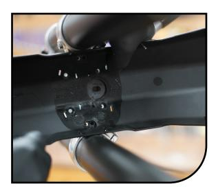
Holding fender up to lower crown, insert machine screw through fender and start threading screw into lower crown boss. Leave fastener loose so the fender position can be adjusted If necessary.
