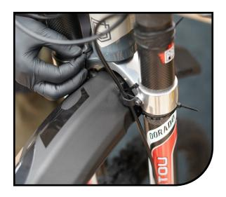
Evenly tighten the zip ties, ensuring the placement of the fender. Before fully tightening zip ties move the head to desired position. Finish final tightening.
