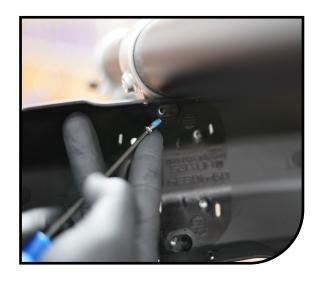
Holding fender up to lower crown, insert machine screw through fender and start threading screw into lower crown boss. Leave fastener loose so the fender position can be adjusted If necessary.
