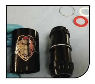
Optional use Air Can Negative Seal Service Tool (172-32193-K001) to ease seal installation. If not available refer to "50 hour Air Can and Piston Service Guide." The flat surface of the tool will help direct the seals into the internal seal glands. Install the quad-ring first.
