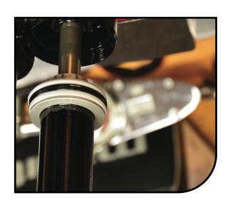
Flip the shock and clamp the eyelet (or clamp across the trunnion faces) into the vise. With the lockout assembly removed, fill the compression assembly with oil. Actuate the lockout lever 5-10x to work air out of the shock.
