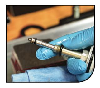
Remove 0-ring (101-600) from the rebound needle. Clean needle with Isopropyl alchohol. Replace the 0-ring (101-600) on the rebound shaft. **DO NOT** grease this 0-ring! Function and assembly is better without grease.
