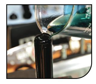
Install the main shaft and piston into the shock damper tube. Add oil if needed to top-off the damper tube once the piston is installed.
