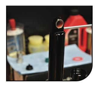
Always ensuring the reservoir is about 2/3 full to prevent air ingestion, repeat step 8 until no air expels from the bleed port. With bleed screw closed and shock in Work mode, the damper should be difficult to compress, with no gap or soft feel at the very beginning of stroke. It may require 5 to 8 cycles to complete this step.
