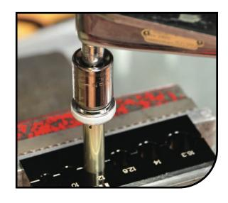
From the bottom of the main piston install a new inner shaft 0-Ring. (PN 101-500-100)
