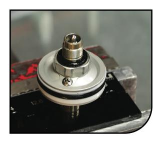
Replace the bottom out bumper 0-Ring (101-1150-0300) above the air piston.
