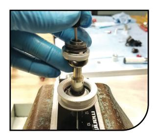
Using an 0-ring pick, remove the white piston ring, and the 0-ring underneath. Install a new 0-ring (PN 101-1810). Install a new piston glide ring (PN 129-30020).
