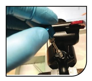
Replace the 0-Ring (101-1600-0180) on the HSC Piston. Replace the 0-Ring (100-018) on the compression cartridge body (above threads at the flange). Grease both 0-Rings.
