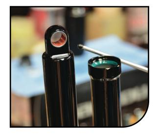
Use a finger to press the IFP down to the specified depth per shock and reservoir size published in Table 2 "IFP Depth."
