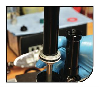
Set the lockout switch to Party Mode. Compress the damper body and note any bubbles rising up in the reservoir.
