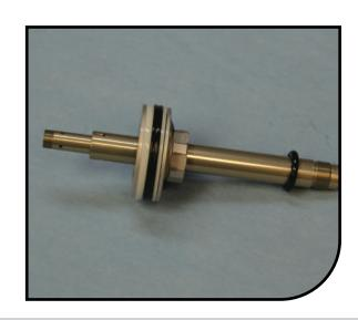
Replace the top-out bumper 0-ring (100-013) on the main shaft that will sit on the main piston.
