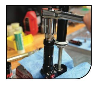
Pressurize the shock IFP to 300psi, test function in a hand dyno.
