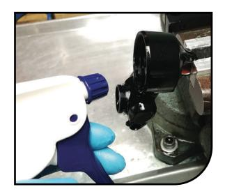
Replace 0-Ring (101-550-100), apply small drop of blue Loctite to the valve stem threads. Reinstall valve stem into top cap torque to 2.3-2.7Nm (20-24 INIbs) Reinstall valve core.
