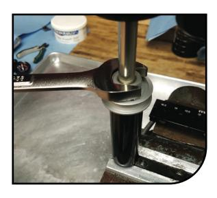
Remove shock from vise and pour oil into catch pan. Cycle shock to allow oil to drain.
