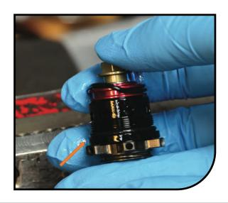
Install the compression assembly into the top cap. Use the compression assembly Pin spanner tool (142-37512-K031) and torque to 5.7Nm (50 in-lb).
