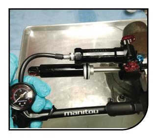
Clean the air can, replace negative spacers, apply grease and install the air can while easing the air piston back-up rings into the air can. Place the shock in a bike or on a hand dyno, compress the shock and thread on the air can to a torque of 10.7Nm (95in-lb).
