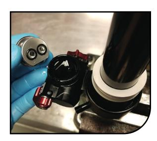
Using a small flathead screw driver, gently pry up to remove the red LSC knob. Be careful when removing this knob, underneath are two detent balls and springs. Pull these out and set aside, remove the 0-ring used to retain the LSC knob.
