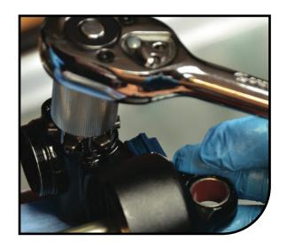
Hold the bottom eyelet in a vise, and place a drip pan under the shock. Using a 21mm wrench, remove the air piston from the damper body.
