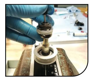
With a small drop of red Loctite, replace the main shock nut on the bottom of the main shaft. Torque to 5nm (45in-lb). \*Excess Loctite can contaminate the assembly)
