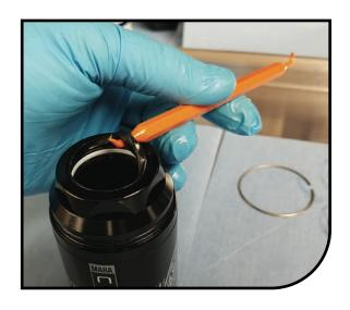
Remove the King Can outer sleeve. Remove the O-rings, remove white back-up ring from the middle groove (Mid-King Can volume setting), and volume spacer rings if used. Thoroughly clean the entire air can with Isopropyl alchohol
