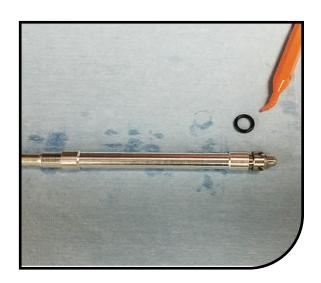
Clamp the main shaft in the 12mm Manitou Clamp Block (PN 172-31464) Remove the piston nut from the shaft with a 16mm socket wrench. Carefully slide the shims and piston onto a small tool like an 0-ring pick or screw driver to preserve the sequence of components. Carefully set aside.
