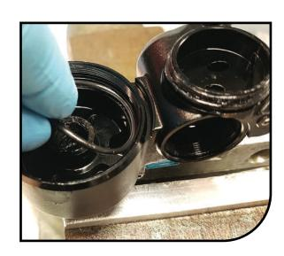
Grease O-rings, reinstall Work/Party assembly into the top cap. Install retention pin, check for full movement of the Work/Party lever by adjusting the depth of the retention pin. Such that the lever flips just past the word "WORK".
