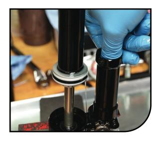
Reinstall the bleed screw while applying a light pressure to the IFP, preventing air entering into the bleed port.
