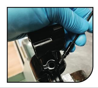
Thoroughly clean topcap, spraying isopropyl alcohol into all ports and passageways. Allow to air dry or blow out with clean compressed air.
