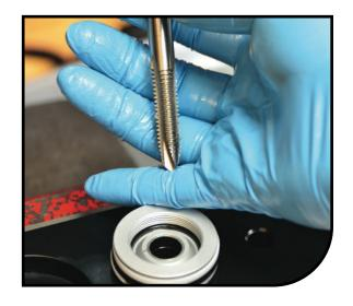
Place the air piston into the first pocket of the service block. Grease the outside of the bullet tool and place it on top of the piston. Use the Air Piston Seal Pusher Tool (PN 172-32189-K001) to install the glide ring onto the air piston.
