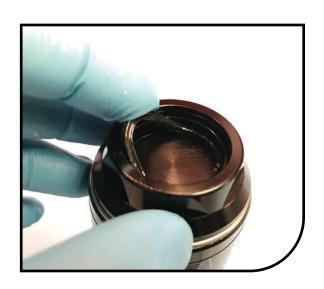
Clamp the shock damper tube in the vise on the eyelet. Fill the damper tube to the top with 3wt Maxima Synthetic damper fluid. (PN 141-34078-K016)\*
