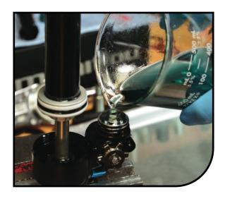
While pushing down firmly to engage the 0-ring thread the reservoir onto the top cap and torque to 9Nm (80 in-lb). Fill the reservoir 2/3 full of oil.
