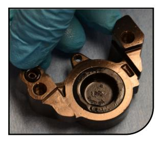
Put the two caliper haves together and install the bridge bolts. Torque the bridge bolts to 170 in lbs +/- 5 in lbs [19.2 N m +/-0.5 N m]
