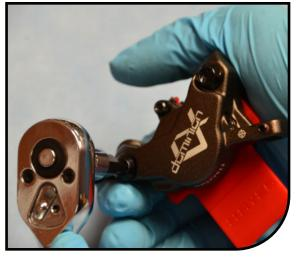
If there is nothing wrong with the hose and the hose fitting, completely remove the caliper hose assembly using a 4mm hex wrench.
