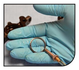
Carefully push the square seal into its seal groove – making sure that the seal is worked into the groove all of the way around and that it is pushed all of the way to the back of the seal groove.
