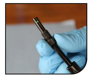
Push the end of the barbed hose insert into the end of the hose. To ensure your bushing is fully seated mark your hose three millimeters down from your cut, push your bushing onto the hose using the side of your workbench until it reaches your mark. Always use a new hose insert/compression bushing.
