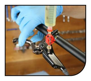
Pull a vacuum at the MC syringe to remove any remaining bubbles.
