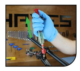
Once there are no air bubbles, push all the DOT 5.1 fluid from the caliper syringe to the master cylinder while flicking the lever several times, and then return the DOT 5.1 fluid back.
