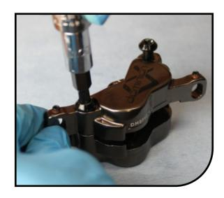
Torque the bridge bolts to 170 in lbs +/- 5 in lbs [19.2 N m +/-0.5 N m]
