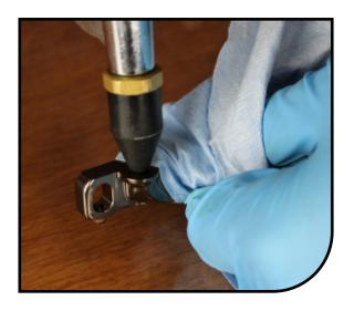
Carefully remove the square seal from inside the piston bore. The replacement kit will consist of a new piston and square seal.
