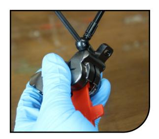
Remove the two bridge bolts - with a T30 Torx wrench. When you remove the two bridge bolts, the caliper will come apart into two pieces. There will be an inner and an outer caliper half and an 0-ring between.
