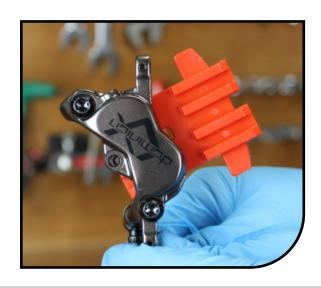
Fill a syringe 3/4 full of DOT 5.1 fluid, eliminate all air from syringe, and close hose clip. Remove the MC bleed screw using a T10 Torx wrench. Place the caliper slightly lower than the MC, and attach to either caliper bleeder.
