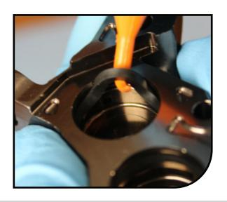
Remove the piston and square seal from the opposing caliper half in the same way.
