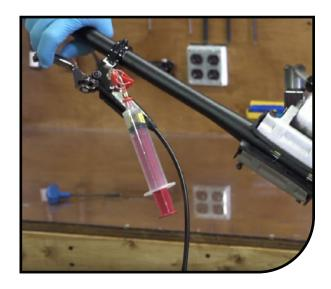
Pull a slight vacuum at the master cylinder to remove any remaining air bubbles and then add positive pressure by slightly depressing the plunger of the syringe.
