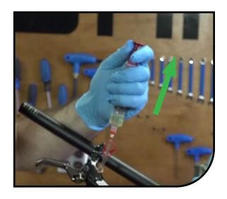
Add positive pressure from the caliper syringe and remove it from the caliper.
