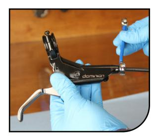
Pull the hose out of the MC. There will be residual fluid in the master cylinder body. Be careful to avoid spilling the fluid.
