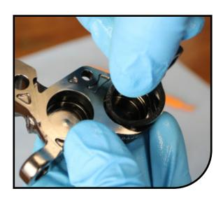
Put a coating of Hayes DOT 5.1 all around the piston as a lubricant, and carefully push the piston into the bore, past the seal, until it seats at the bottom of the bore. The piston should push in easily, if it doesn't, take the piston out and again push the square seal all of the way to the back of the groove and then try again.
