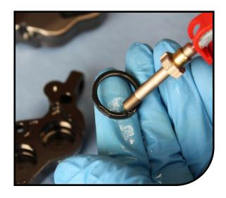
Carefully push the square seal into its seal groove – making sure that the seal is worked into the groove all of the way around and that it is pushed all of the way to the back of the seal groove.
