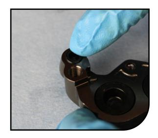
Put the two caliper haves together and install the bridge bolts.
