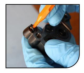
Remove the pistons from the caliper with pressurized air. Avoid chipping the piston. Ensure bleed plug is installed, angle the caliper so the piston is facing downward, then direct pressurized air thru the hole that connects the two halves together. This will force the first piston out of the caliper halve. Be sure you are blowing the piston into a clean rag. The air pressure will force the piston out at a high rate of speed. Place a rag and you thumb over the
