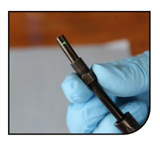
Push the end of the barbed hose insert into the end of the hose. To ensure your bushing is fully seated mark your hose three millimeters down from your cut, push your bushing onto the hose using the side of your workbench until it reaches your mark. Always use a new hose insert/compression bushing.
