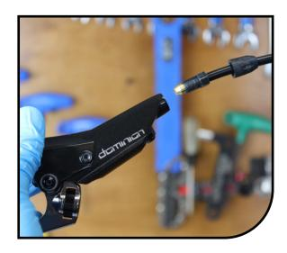
Using an 8mm crows foot, torque the hose nut to  $70 \pm 5$  in lbs [7.9 $\pm$ 0.5 N m]
