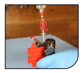
Fill second syringe 1/4 full of DOT 5.1 fluid, eliminate all air from syringe, and close hose clip. Remove the MC bleed screw using a T10 Torx wrench and attach to the MC bleeder.
