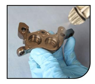
Wipe down each part to remove the residue. Then use compressed air to blow dry and remove all of the remaining dirt, etc. For both caliper halves, be sure to blow compressed air through both the bleeder hole and the transfer port, and all around the square seal groove. Take extra care to get the square seal grooves free of any hair, dirt, scratches, etc. that could cause the caliper to leak.
