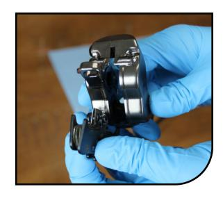
Fill space in caliper with dummy pads and bleed block or something else. If nothing is available then be careful during bleed not to advance the pistons.
