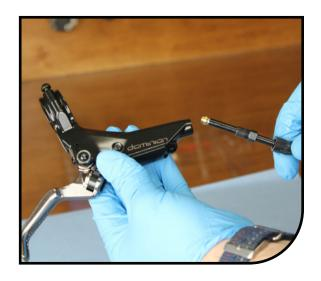
A new hose insert/compression bushing combination will be needed each time the hose is re-installed.
