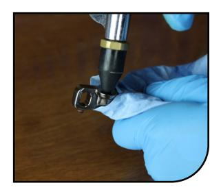
Clean all of the parts. Then rinse each part with mild soap and water. Be sure to clean the caliper through all of the holes.
