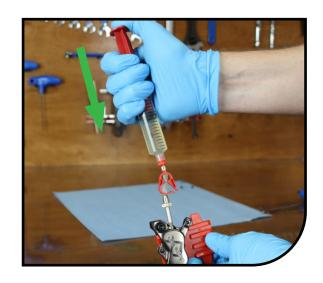
Push DOT 5.1 fluid from caliper syringe to MC syringe while flicking the lever several times, then return.
