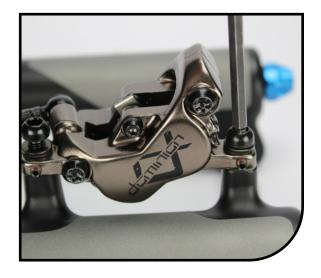
If there is nothing wrong with the hose and the hose fitting, completely remove the caliper hose assembly using a 3mm hex wrench.
