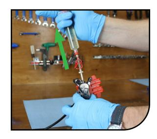
Push all DOT 5.1 fluid from caliper syringe to MC syringe, then return. Repeat until no bubbles are found.
