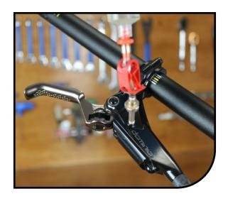
Open both syringe hose clips and pull a small vacuum at the caliper syringe to pull any air that was introduced.
