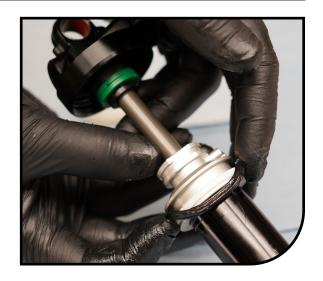
Ensure the air piston quad ring is not twisted and push it tight against the glide ring, making a space for the split glide ring.
