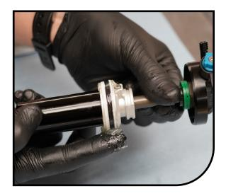
Install foam ring bumper and spacer onto damper body.
