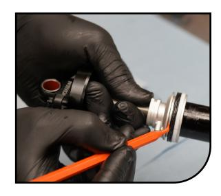
10 Install the split glide ring onto the air piston.
