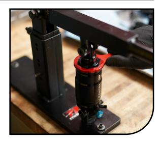
Pressure should be increased in increments of 75psi. With the shock pump attached cycle the shock a few times past the sag point to balance the positive and negative chambers. The first few cycles may feel firm / top out, this is normal until the negative is balanced. When the desired air pressure is achieved, cycle the shock and recheck the pressure.
