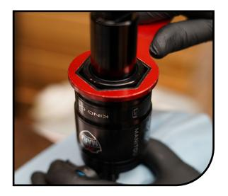
Remove air can, foam ring bumper, and spacer.
