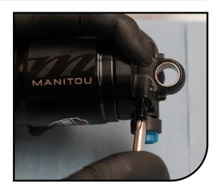
Clamp upper eyelet of shock in vise. If Trunnion shock, clamp on trunnion mounts. (Use soft jaws to not damage the shock)
