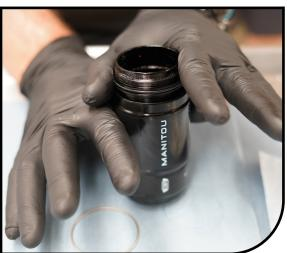
Note orientation of Spacers in the positive and negative air chambers. Do not alter spacer orientation unless an air volume tuning change is desired.
