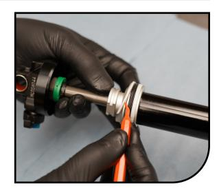
Remove the air piston quad seal. Inspect white glide ring. replace if wear is found. To remove glide ring must be cut. Installation requires sizing before quad ring is installed. Clean the white glide ring and air piston with isopropyl alchohol.
