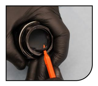
To make air can seal installation easier use the Air Can Seal Install tool, Manitou part number 172-32193-K001.
