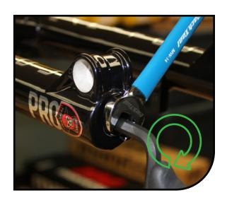
Unscrew air cap and attach shock pump. Depress pressure bleed button until pump reads "Zero".
