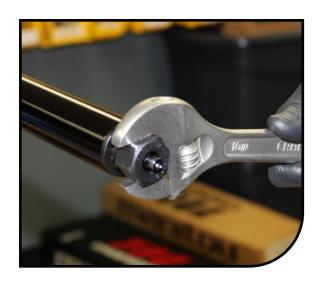
Remove Air Spring Assembly, clean with isopropyl, Inspect seal for damage. Replace air piston seal 141-32155-K012 (Pro/Exp) or 141-32156-K011 (Comp). If Travel change is need see page 34 before moving on.
