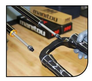
Using a downhill tire lever or similar tool, gently pry the dust seals out of the casting.
