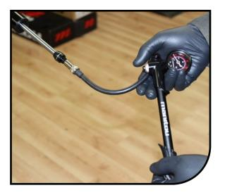
Using a 2mm Hex wrench remove the screw of the red "LO-SPEED" MC2 knob.
