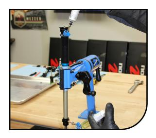
Closing the bleed hose clamp on both syringes cycle the damper SLOWLY to draw air to the top of the damper. Open bleed hose clamps and repeat step 10 until no air bubbles are present in oil drawn into upper syringe.
