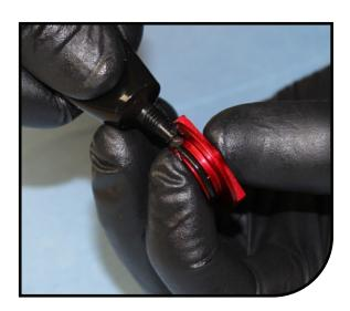
Clean fork and use a shock pump to set to desired pressure. Lightly pull the casing away from the CSA as you add air.
