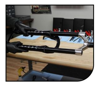
Insert 14cc of semi-bath (85-0022) into each casting leg. Once the semi-bath is in the legs slide the casting the rest of the way onto the stanchion assembly until the damper and spring shaft adapters pass thru the end of the casting. Some manual alignment may be needed.
