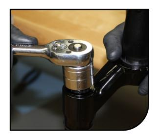
Remove damper assembly from the stanchion. Inspect damper piston seal for any damage.
