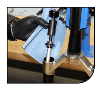
Tip out used damper oil from top of stanchion into drain pan. Cycle damper shaft serval times to cycle out old oil from damper.
