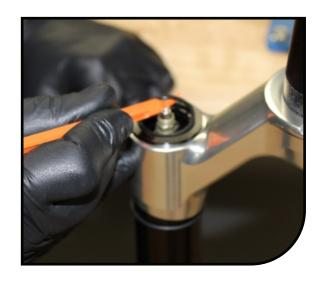
Use a standard cassette tool and 1" socket to unthread the damper top-cap from the stanchion.
