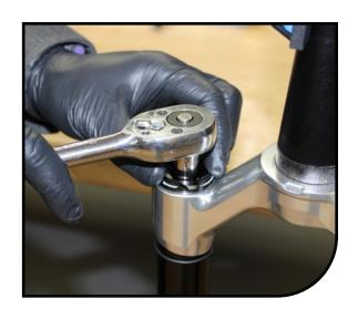
Remove the v-seal that was under the black "HI-SPEED" adjustment knob.
