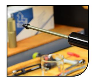
Fully extend the damper shaft.
