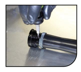
Install Damper cartridge into stanchion. Using standard cassette lock-ring tool Torque to 200-220 LB-in [22.6-25 Nm].
