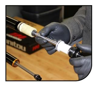
Once the air spring assembly is removed clean the inside of the stanchion with isopropyl alcohol and a lint free towel (Be careful to not scratch the inner surface of the stanchion). Inspect the inside and outside of the stanchion for scratches or other damage.
