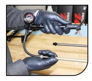
Fully extend the damper shaft.
