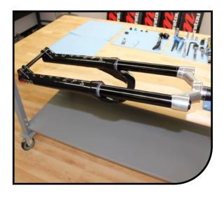
Insert 14cc Mattoc / Circus Pro, 7cc JUnit 34 of semi-bath (85-0022) into each casting leg. Once the semi-bath is in the legs slide the casting the rest of the way onto the stanchion assembly until the damper and spring shaft adapters pass thru the end of the casting. Some manual alignment may be needed.
