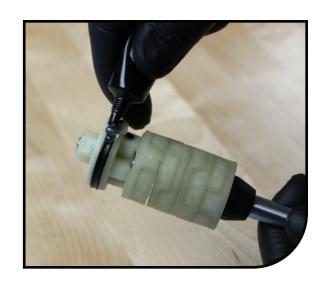
Add Slickoleum<sup>™</sup> grease to the stanchion threads before inserting the air spring assembly. Spread grease across entire thread surface.
