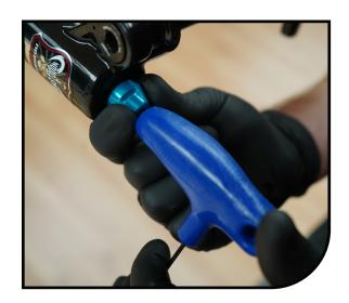
Hold lock-nut with 14mm end wrench for Pro & Expert, or a 19mm end wrench for Comp. Insert a 8mm Hex wrench into the end of the rebound rod and loosen clockwise until rebound rod disengages from the lock-nut.
