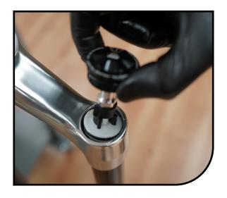
Install IVA cap into stanchion. Torque 12 to 200-220 LB-in [22.6-25 Nm] using a 24mm socket.
