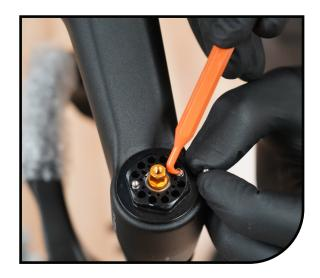
Use 24mm socket to unthread the damper top cap from the stanchion.
