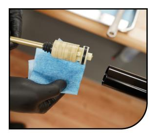
Once the air spring assembly is 6 removed clean the inside of the stanchion with isopropyl alcohol and a lint free towel (Be careful to not scratch the inner surface of the stanchion). Inspect the inside and outside of the stanchion for scratches or other damage.
