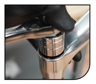
Remove damper assembly from the 5 stanchion. Inspect damper piston seal for any damage.
