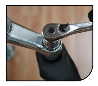
Pull IVA assembly straight out, Clean with isopropyl, Inspect seal for damage. If needed replace IVA piston seals.
