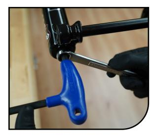
Remove casting from fork. It is 5 recommended this be done over a drain pan as the lower casting contains semi-bath oil. Allow oil in casting to drain out before continuing to next step.
