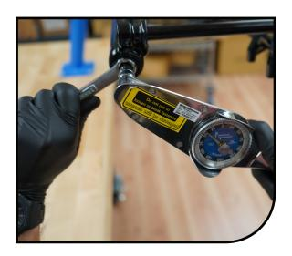
Install the rebound knob using a 2mm 6 Hex wrench. Add a small drop of blue Loctite to the screw before installation to prevent the screw from backing out during riding.
