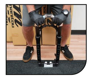
With the fork fully extended add oil 3 to the height of 75mm for VTT6 and 87mm for ABS+ measured from the top of the stanchion.
