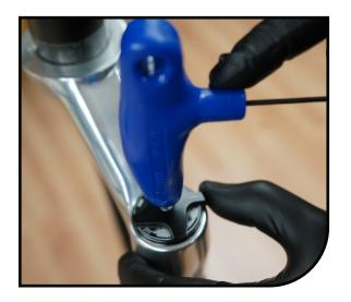
Use a non-marring pick or pliers with non-marring barrier to remove the black VTT knob by lifting straight up.
