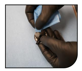
**Option:** ABS+ Install springs and ball bearings into ABS+ top cap. A small dab of grease on top of the spring can help hold the ball bearings in place.
