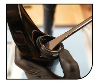
Remove old foam wiper rings. Clean Casting. Thoroughly saturate new foam rings with semi-bath fluid and install into fork casting.
