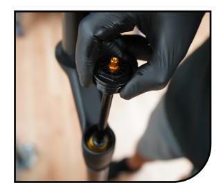
Tip out used damper oil from top 5 of stanchion into drain pan. Cycle damper shaft serval times to cycle out old oil from damper.
