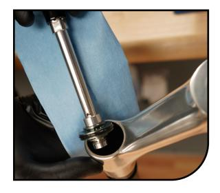
Tip out used damper oil from top 6 of stanchion into drain pan. Cycle damper shaft serval times to cycle out old oil from damper.
