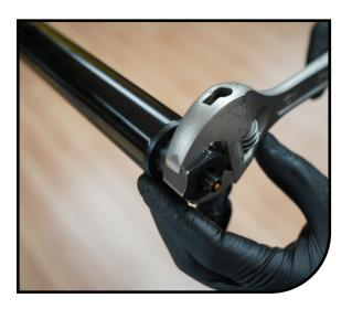
Remove Air Spring Assembly, clean with isopropyl, Inspect seal for damage. Replace air piston seal 141-32155-K012 (Pro) or 141-32156-K011 (Comp). If Travel change is needed see page 24 before moving on.
