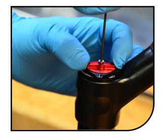
Use a non-marring pick or pliers with non-marring barrier to remove the red "LO-SPEED" compression knob by lifting straight up.
