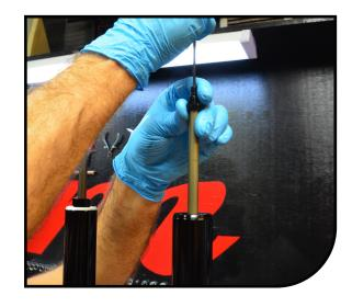
Remove Air Spring Assembly, clean with isopropyl, Inspect seal for damage. Replace air piston seal (141-36713-K027). If Travel change is need see page 26 before moving on.
