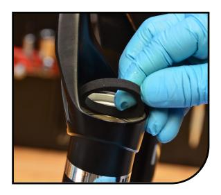
Remove springs from outer lip of new leg seals. Clean casting seal press area with Isopropyl alcohol. Using the Manitou 37mm Seal Press press in the dust seals. Reinstall springs onto seals.
