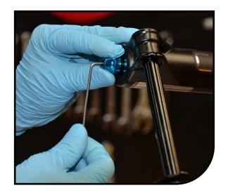
Hold lock-nut with 14mm box end wrench. Insert a 8mm Hex wrench into the end of the rebound rod and loosen clockwise until rebound rod disengages from the lock-nut.
