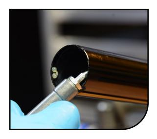
Install air spring assembly into stanchion. Using a 26mm crow's foot and Manitou cassette tool **OR** 1" Socket and Standard cassette tool torque to 20-25 in-lb [2.3-2.8 Nm]. If rod is bottomed attach shock pump to valve and draw the rod out until fully extended.
