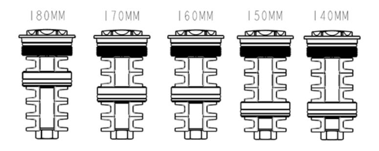
The air volume is modified by removing the clip-on spacers from the IVA shaft moving the piston into the desired location and reassembling the clip-on spacers to secure the piston on the IVA shaft.
