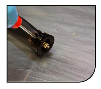
Attach M5x0.8 Luer lock fitting to both syringes (141-30694-K020). Fill one syringe with 5wt Damper oil (85-0023).
