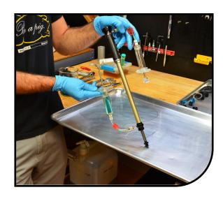
Holding the damper end-cap up-right in vise simultaneously compress the filled syringe and retract the empty syringe to remove air from the damper. Refill the syring as needed until oil is drawn into the upper syringe.
