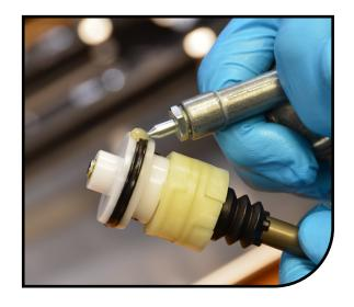
Add Slickoleum<sup>™</sup> grease to the stanchion threads before inserting the air spring assembly. Spread grease across entire thread surface.
