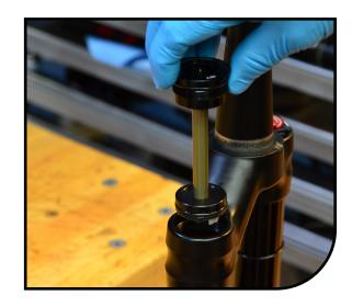
Invert the fork and use Manitou cassette tool with adjustable wrench to unthread the air spring assembly from the stanchion.OR depress valve on end of comp-rod with 2mm hex and stroke rod to bottom. Slide standard cassette lock-ring tool over threaded adapter and unthread the air spring assembly from the stanchion.
