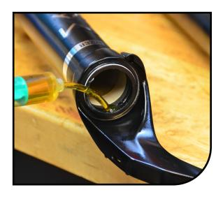
Make sure the spring shaft is fully extended and air chamber is filled with air (60PSI).
