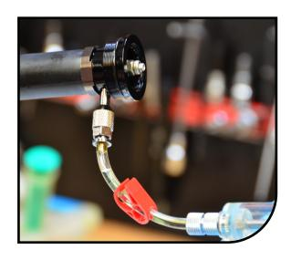
Attach the empty syringe M5x.8 adapter to top-cap bleed port. Remove bleed-screw from damper end-cap and attach the filled syringe M5x.8 adapter to end-cap bleed port.
