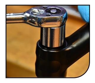
Remove damper assembly from the stanchion. Inspect damper shaft and bladder for any damage.
