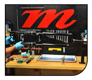
Insert 21cc of semi-bath (85-0022) into each casting leg.
