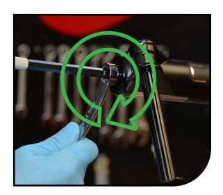
Unscrew air cap and attach shock pump. Depress pressure bleed button until pump reads "Zero". Depress Schrader Valve a few times with 2mm hex wrench to ensure all air is released.
