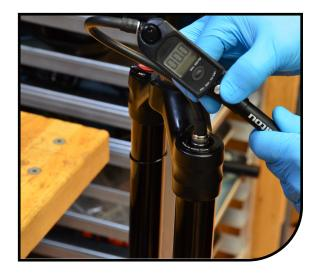
Mezzer Pro: Using a standard cassette tool and 1" socket loosen IRT cap until threads are free from leg.
