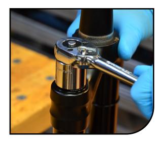
Mezzer Pro: Pull IRT assembly straight out, Clean with isopropyl, Inspect seal for damage. If needed Replace IRT piston seals (141-36713-K026).
