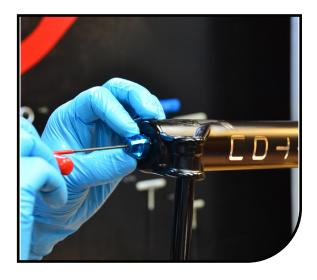
Thread the other lock-nut onto the spring shaft adapter. Holding the lock-nut with a 14mm box wrench, use an 8mm socket tighten the compression rod adapter to 5,7-6,4 N-M [50-57 LB-IN] by turning them **counter-clockwise**. Do not overtighten, doing so can damage the threads.
