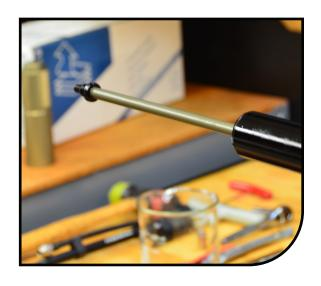
Fully extend the damper shaft.
