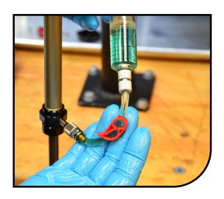
Fully extend damper shaft and add oil from bottom syringe until bladder is slightly expanded. Closing the bleed hose clamp on both syringes remove cartridge from vise. Lay cartridge flat on bench. Remove lower syringe and replace bleed screw. Some oil may discharge from bleed port when removing syring. Remove upper syringe and replace bleed screw.
