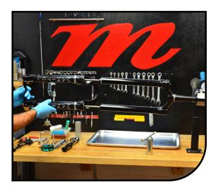
Insert 21cc of semi-bath (85-0022) into each casting leg.
