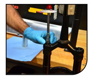
Lubricate o-ring seal on red "LO-SPEED" adjustment knob with Slickoleum™ Grease an install onto adjuster hex. With a 2mm hex, thread on the screw and torque to 4-6 in-lb [0.5-0.7 Nm] Note: Be sure to hold the knob still while installing the screw. The damper adjuster may be damaged if the knob is over torqued.
