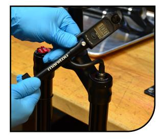
Attach a shock pump and inflate main air chamber to 60PSI.
