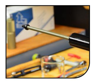
Fully extend the damper shaft.
