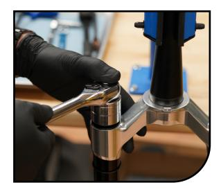
Pull damper shaft to full extension. Remove bleed-screw on side of top-cap. Place damper top-cap over catch pan. Cycle damper shaft several times to cycle out old oil from damper.
