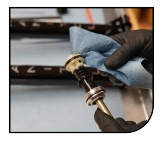
Liberally apply Slickoleum<sup>™</sup> grease to the piston seal, outer piston surface, and spring shaft. Add 3cc's of Slickoleum<sup>™</sup> grease to the top of the air piston.
