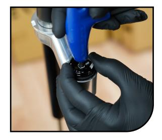
Holding the outer surface of the cable stop, lift the entire remote knob assembly out of the top-cap. The remote knob may spin when it disengages from the adjuster; this is normal. Further disassembly of the knob assembly is not needed.
