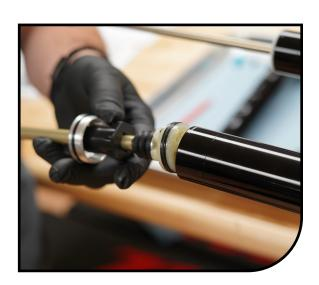
Once the air spring assembly is removed clean the inside of the stanchion with isopropyl alcohol and a lint free towel (Be careful to not scratch the inner surface of the stanchion). Inspect the inside and outside of the stanchion for scratches or other damage.
