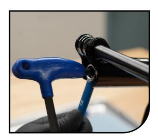
Unscrew air cap and attach shock pump. Depress pressure bleed button until pump reads "Zero". Depress Schrader Valve a few times with 2mm hex wrench to ensure all air is released.
