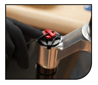
With a 11mm socket, unthread the exposed nut and remove the black "VTT" adjustment knob.
