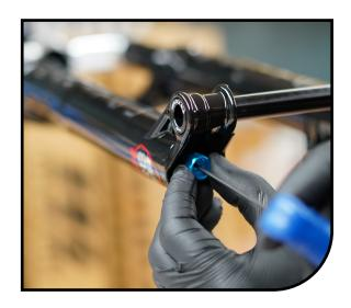
Thread the other lock-nut onto the spring shaft adapter. Holding the lock-nut with a 14mm box wrench, use an 8mm socket tighten the compression rod adapter to 5,7-6,4 N-M [50-57 LB-IN] by turning them counter-clockwise. Do not overtighten, doing so can damage the threads.
