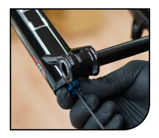
Hold lock-nut with 14mm end wrench. Insert a 8mm
