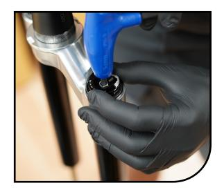
Insert the remote cable thru the cable stop housing and along the knob track. Using a 2mm hex partially insert a set-screw into the first threaded hole on the remote knob. Tension the cable then torque the set screw to 0.5-0.7 N-M [4-6 lb-in].
