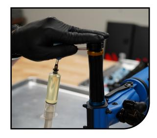
Fully extend damper shaft and add oil from the syringe until bladder is slightly expanded. Closing the bleed hose clamp on the syringe remove cartridge from vise.
