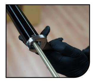
Remove Air Spring Assembly, clean with isopropyl, Inspect seal for damage. Replace air piston seal 141-32155-K012. If Travel change is need see page 27 before moving on.
