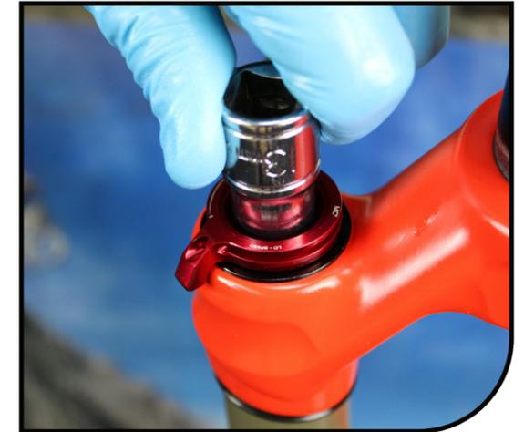
**8** Place high speed and HBO knob assembly onto the red low speed adjustment knob. Tighten down screw with 2mm Hex wrench.
