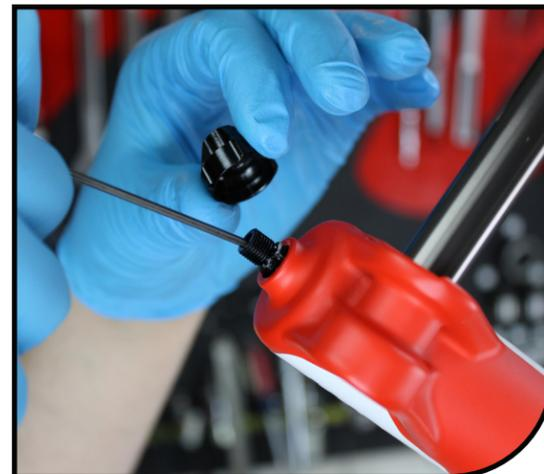
**4** Using the Mattoc 8mm Thin Wall Socket, turn the compression rod **clockwise** until compression rod is disengaged from the casting threads.
