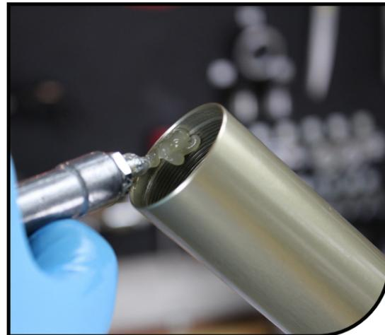
**8** Install air spring assembly into stanchion. Using a 26mm crow's foot and Manitou cassette tool, torque to spec.
