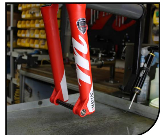
**6** Using a downhill tire lever or similar tool, gently pry the dust seals out of the casting.
