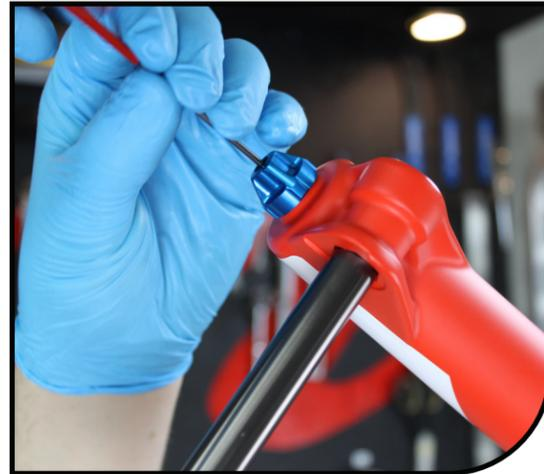
**2** Insert a 8mm Hex wrench into the end of the rebound rod and loosen **clockwise** until rebound rod disengages from the casting threads.
