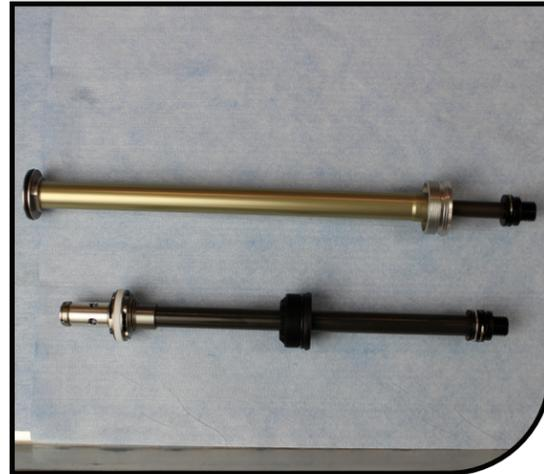
**9** Use a 26mm crow's foot, Manitou cassette tool, and torque wrench to install the rebound damper assembly.
