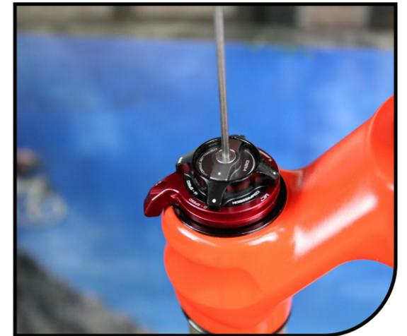
**9** Clean fork and use a shock pump to set to desired pressure. Lightly pull the casing away from the CSA as you add air. Pressure chart below for reference.
