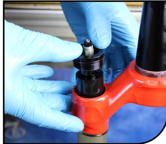
**5** Using a crow's foot, Manitou cassette tool, and torque wrench, tighten down the MC2 at a torque of 60–80 in lb [6.8–9.0 N m].
