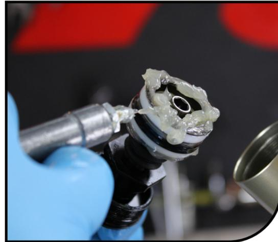
**7** Add Slickoleum™ grease to the stanchion threads before inserting the air spring assembly. Spread grease across entire thread surface.
