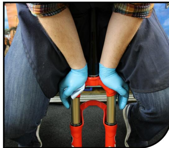
**3** Pour additional 5wt fork oil into the damper leg until the oil height (space from the top of the damper leg to the top of the oil) is set at the proper level. See following page for the correct oil height depending on compression damper type and fork travel. An oil height setting tool used for motorcycle forks similar to the one pictured makes this job easier.
