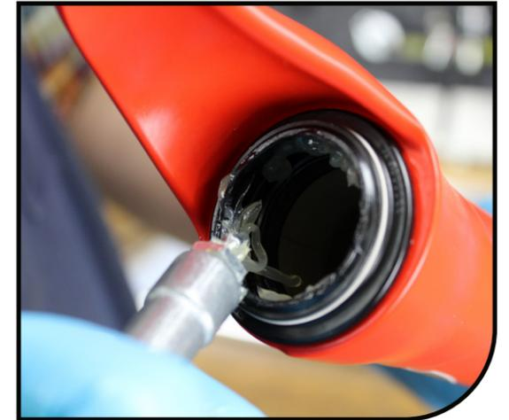
**2** Fill the air chamber with air (60PSI). This will extend the air spring assembly and make casting installation easier.
