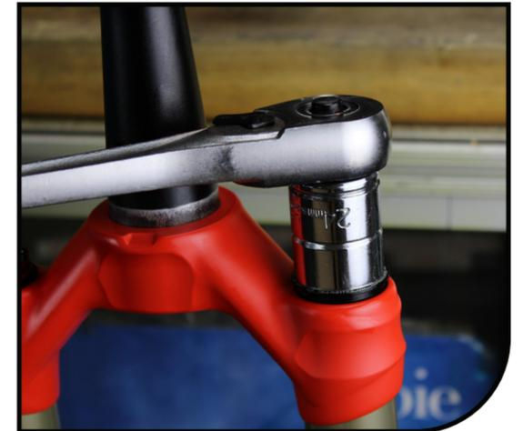
**10** Attach a shock pump and inflate air leg to 60PSI. This will aid in installing the casting later.
