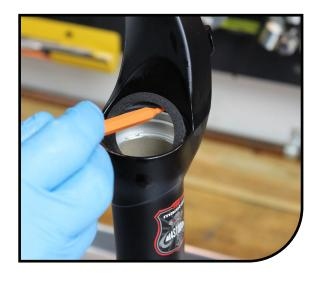
Remove springs from lip of dust seals. Clean seal area with Isopropyl alcohol. Using the Manitou 34mm Seal Press or large socket press in the dust seals. Reinstall springs onto seals.
