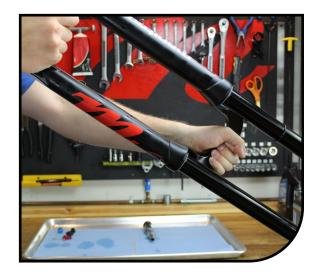
Insert 7cc of semi-bath into each casting leg. Once the semi-bath is in the legs slide the casting the rest of the way onto the stanchion assembly.
