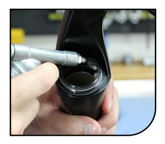
Make sure the air chamber is filled with air (60PSI). This will extend the air spring assembly and make casting installation easier.
