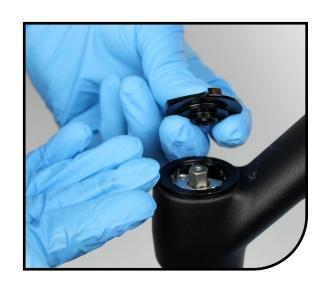
Use a standard cassette tool, 1" socket, and socket wrench to unthread the compression damper assembly from the stanchion.
