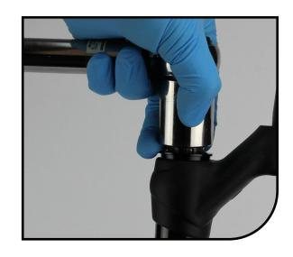
Place the silver spacer onto the MC2 damper, flat side facing up.
