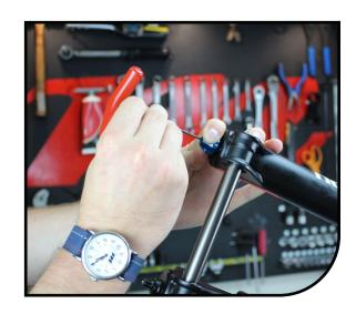
Insert a 8mm Hex wrench into the end of the rebound rod and loosen **clockwise** until rebound rod disengages from the casting threads.
