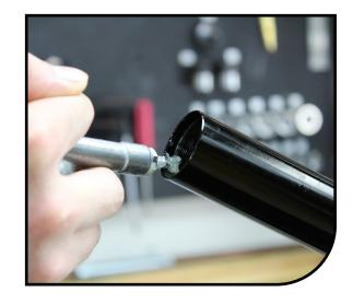
Install air spring assembly into stanchion. Using a 26mm crow's foot and Manitou cassette tool, torque to 60-80 in lb [6.8-9.0 N m].
