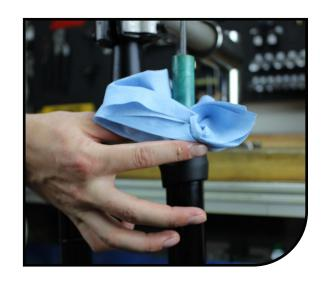
Liberally grease the piston quad seal and outer surface with Slickoleum™ grease. Add 8cc's of Slickoleum™ grease to the top of the air piston.
