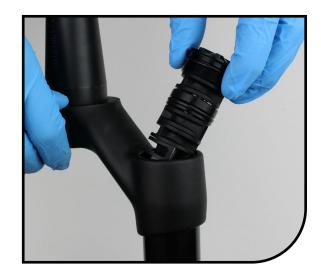
Invert the fork and use Manitou cassette tool with adjustable wrench to unthread the air spring assembly from the stanchion.
