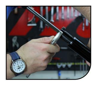
Remove Air Spring Assembly, clean with isopropyl, and regrease.
