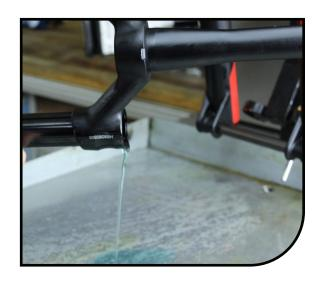
Using a Manitou cassette tool and adjustable wrench, unthread the rebound damper assembly from the fork stanchion.
