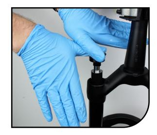
Using the standard cassette tool, 1" socket, and torque wrench to tighten down the VTT at a torque of 220 in lbs [25 N m].
