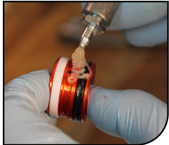
7 Install new, greased air piston into the top of the stanchion and push it down past the threads.
