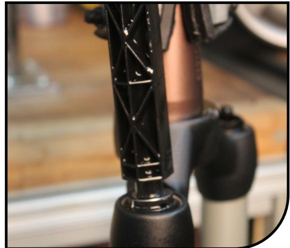
5 If installing an ABS+ damper use a 24mm socket and torque wrench, tighten the damper to 60–80 in lbs [6.8–9.0 NM]. If installing a Kwik Toggle damper use a 1" socket or crow's foot, the Mattoc Cassette tool and a torque wrench to tighten down the damper to the same torque specification.
