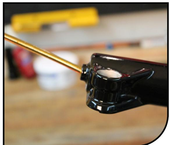
6 Using an 8mm Allen wrench tighten the rebound damper rod and air spring assembly to 35–40in lbs [3.95–4.5 Nm] by turning them counter-clockwise. Do not overtighten, doing so can damage the end of the rods.
