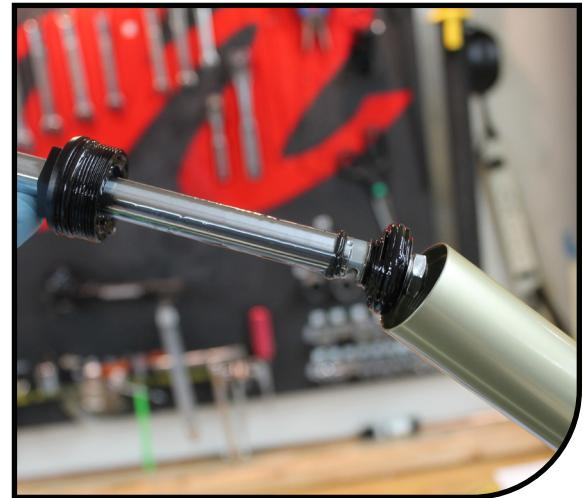
7 Install rebound damper into stanchion. Using a 22mm crow's foot and torque wrench, tighten the rebound damper assembly end cap to 80-100 in lbs [9.0-11.3 NM].
