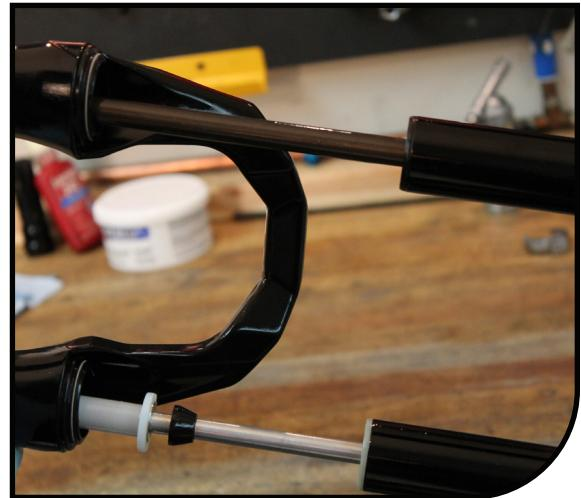
5 Insert 15cc's (15ml) of semi-bath into each casting leg. Once the semi-bath is in the legs slide the casting the rest of the way onto the stanchion assembly.
