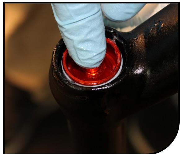
8 Add 8cc's of Slickoleum™ grease to the top of the air piston.
