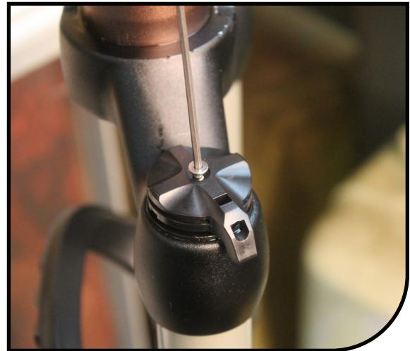
8 Clean fork and use a shock pump to set to desired pressure. Pressure chart below for reference.
