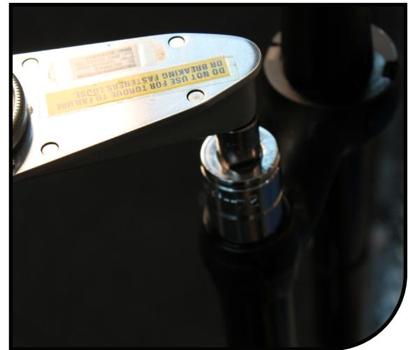
10 Install air spring assembly into stanchion. Using a 22mm crow's foot, tighten assembly end cap to 80-100 in lbs [9.0-11.3 NM].
