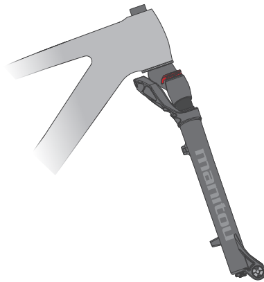
Reverse Arch does not affect frame clearance
