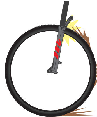
Reverse Arch shields the seals from debris
