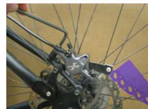
(Fig. 3) Centering the caliper with Feel 'R Gauge in place
