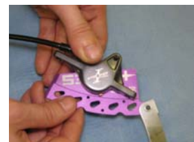
(Fig. 5) Testing for proper caliper retraction using the thick edge of the tool.
