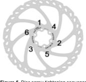
Figure 5. Disc screw tightening sequence
