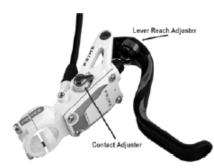
Figure 4. Contact (dead stroke) and lever reach adjustment.
