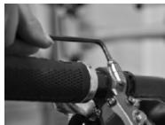
Figure 1. Tighten the side of the clamp with the Prime logo until there is no gap
