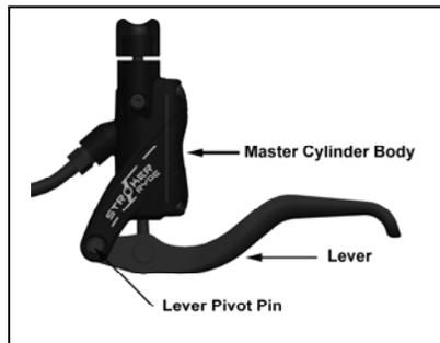
Figure 1. Location of lever pivot pin.
