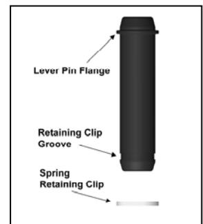
Figure 4. New lever pivot pin features.
