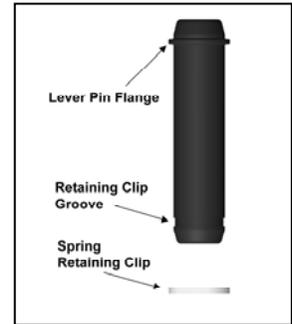
Figure 4. New lever pivot pin features.
