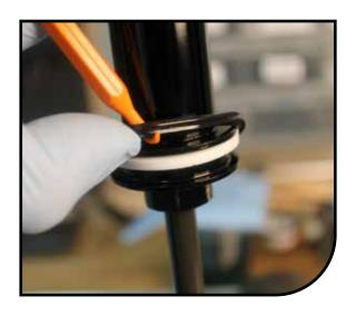
To easily remove the air piston glide ring first use a small side cutters to cut the ring about halfway through.
