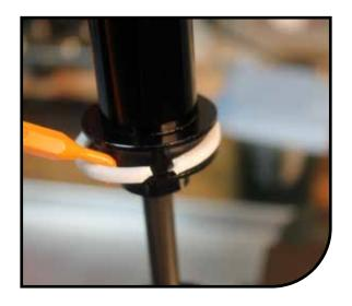
First we will install the new air piston glide ring. This ring can be difficult to install so here is a way to make it easier. Take a lanyard or similar item and cut it into two strips.
