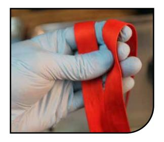
6 Loop the lanyard strips around the air piston glide ring.
