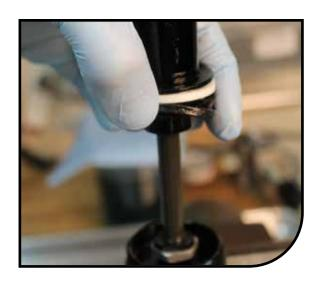
Ensure the air piston quad ring is not twisted and push it tight against the glide ring, making a space for the split glide ring.
