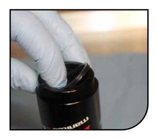
Install the air can glide seal into the same groove as the quad ring. It will sit on top of the quad ring.
