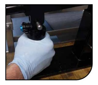
Remove shock from tester or frame and pull air can off of the shock.
