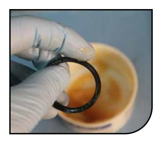
Install the air piston quad ring onto the air piston.
