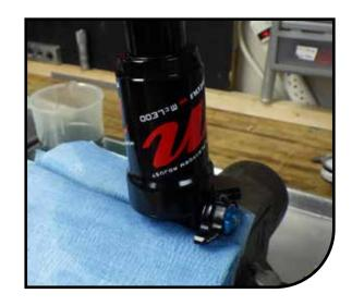
Using an air can wrench or similar tool loosen the air can 2-3 turns. Do not remove the air can completely. The negative air pressure will cause the air can to pull away from the top cap threads. Removing the air can without slightly compressing the shock can damage the threads.
