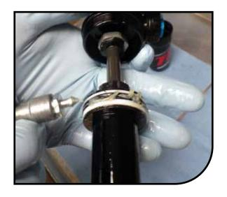
Install foam ring onto damper body.
