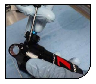
Clamp the top cap of the shock in a vise. Be careful to clamp below the set screw to avoid damaging it.
