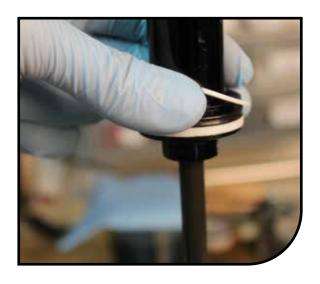
Remove the air piston quad seal.
