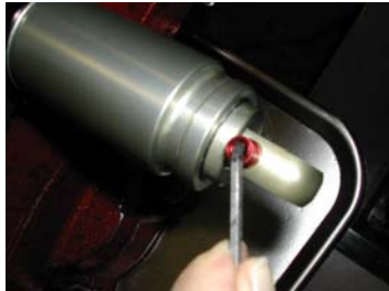
Schrader Removal Using 3mm Hex Wrench
