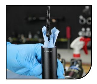
Apply blue Loctite<sup>™</sup> to the threads of the new cartridge damper.
