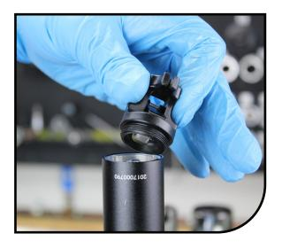
Use the Jack Spanner tool to unthread the cartridge from the outer tube.
