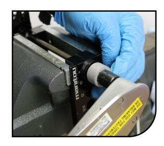
Thread air cartridge pushrod cap into top of stanchion. Torque to 60 in lbs [6.7 N m]
