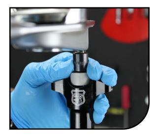
Install seat clamp. Be sure the white arrow on the top plate is pointing to the front of the post.
