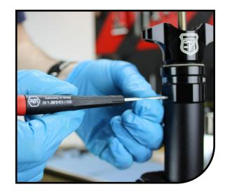
Apply Loctite<sup>™</sup> to air cartridge pushrod threads.
