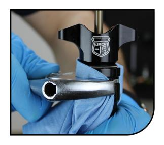
Pull stanchion up and remove from outer tube.
