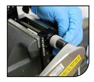
Thread air cartridge pushrod cap into top of stanchion. Torque to 60 in lbs [6.7 N m]
