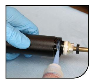
Slide collar down and thread onto the lower tube. Torque to 43 in lbs [58.30 N m]
