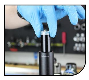
Thoroughly clean the inside of the outer tube with lint-free rags and isopropyl alcohol.
