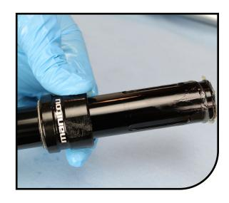
Assemble new keys as shown. Grey key on top of black key.
