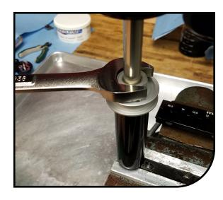
Place the main shock shaft 18 into the 12mm Manitou clamp block. Using an eyelet tool such as a pin wrench or an adjustable wrench accross the flat turn the top cap counter clockwise to release the top cap from the main shock shaft.
