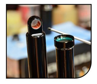
Use a finger to press the IFP 14 down to the specified depth per shock and reservoir size published in Table 2 "IFP Depth."
