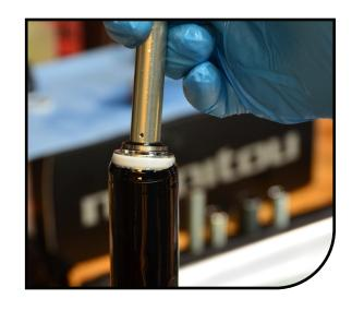
Remove the bleed screw on the air piston so that air can escape while the air piston is threaded on to the damper tube. Torque the air piston to 26Nm (230in-lb). Replace the bleed screw.
