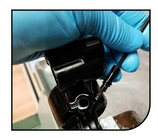
Thoroughly clean topcap, spraying isopropyl alcohol into all ports and passageways.
