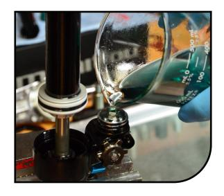
While pushing down firmly to engage the O-ring thread the reservoir onto the top cap and torque to 9Nm (80 in-lb). Fill the reservoir 2/3 full of oil.
