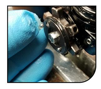
Reinstall LSC knob by pushing straight down to not disrupt the detent balls.
