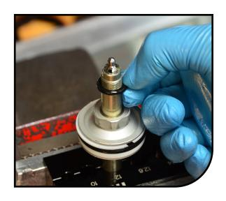
Install the bottoming shims or 16 spacers. \*Some shocks may have a 2.5mm plastic spacer or a 5mm aluminum spacer.\*
