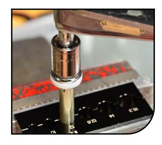
From the bottom of the main 12 piston install a new inner shaft O-Ring. (PN 101-500-100)
