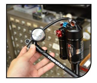
Refer to Mara Set-up guide for 20 air can pressure.(See Below)
