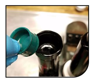
The shock's lock-out piston will be visible at this point, carefully remove this assembly and set aside on a lint-free rag. Be sure to account for the rubber face seal which may still be in the top cap when assembly is removed.
