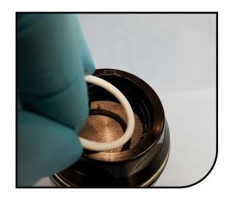
Install the wiper seal, with the narrow lip facing externally.
