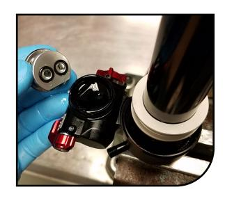
driver, gently pry up to remove the red LSC knob. Be careful when removing this knob, underneath are two detent balls and springs. Pull these out and set aside, remove the O-ring used to retain the LSC knob.
