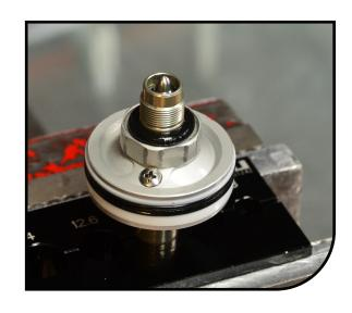
Replace the bottom out bumper O-Ring (101-1150-0300) above the air piston.
