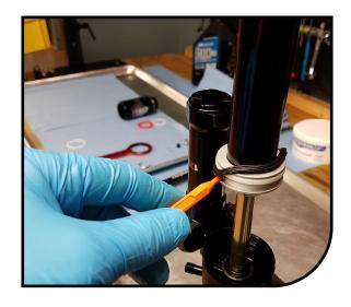
A small side-cutter can be used to first partially cut the large piston ring, then break it to remove. Be careful not to damage the groove.
