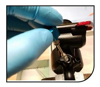
Replace the O-Ring (101-1600-0180) on the HSC Piston. Replace the O-Ring (100-018) on the compression cartridge body (above threads at the flange). Grease both O-Rings.
