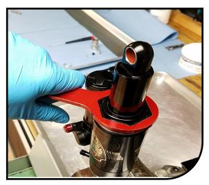
Place shock in a hand dyno or in a bicycle frame, slightly compress the shock. At this point unthread the air can fully.
