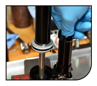
Reinstall the bleed screw 15 while applying a light pressure to the IFP, preventing air entering into the bleed port.
