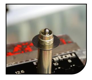
Hold the main shaft in the vise using Manitou clamp block tool (172-31464). Thread the top cap onto the main shaft and torque to 11.3Nm (100in-lb)
