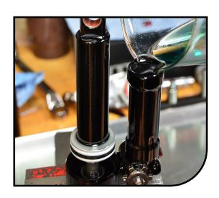
The large cup side of the SKF IFP will be facing up (towards the gas charge side). Use 1 edge, and "scoop" the shallow face of the piston into the oil, allowing the small air pocket to clear before submersing. Stop when the leading edge of the IFP is engaged on the primary inner diameter of the reservoir below the threads.
