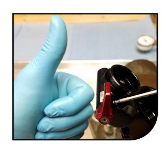
Apply a dab of grease to the O-ring, ramped surface and thread on the rebound adjuster. Insert into top cap, rotate counter-clockwise to engage the left handed thread. Turn until it lightly bottoms. Reinstall spring and detent ball.
