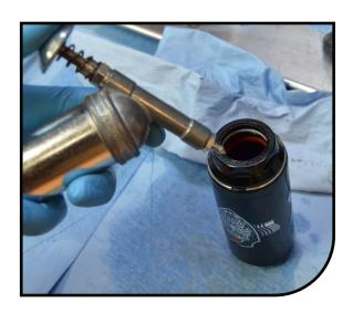
Clamp the shock damper tube in the vise on the eyelet. Fill the damper tube to the top with 5wt damper fluid. \*For cold weather use Maxima Synthetic All Temperarture 3wt fork oil. (PN 141-34078-K016)\*
