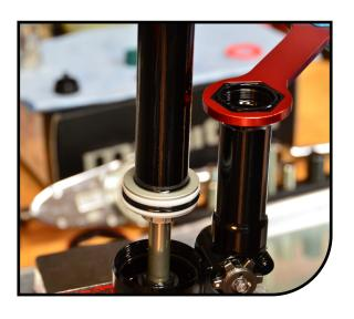
Set the Lockout to Party Mode. Slowly compress the damper body about 1/2 way or until bubbles stop coming up in the reservoir. Compressing slowly helps reduce atomization of the bubbles, allowing them to rise out more quickly. Fully extend the damper body.
