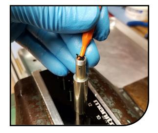
If the service warrants replacement of bushings within the air piston, use a ½-13 UNC bottoming tap and the Manitou clamp block to remove the bushings. (See Manitou Air Piston Bushing and Seal Tool instructions for information)
