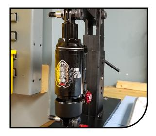
Remove air can, bumper, and 5 spacers (if present). These may remain in the air can, locate and save for later reassembly.
