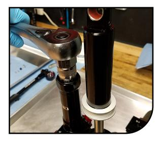
Place a catch basin under the 12 shock to catch oil. Use the air can / reservoir wrench (PN 142-37512-K033) to unthread the shock reservoir. (Alternative: use a 30mm wrench)
