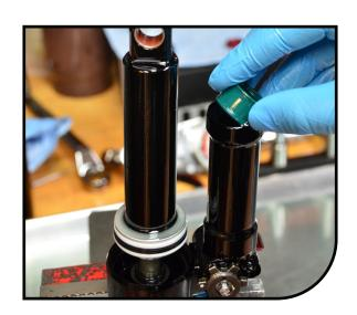
Ensure damper is fully extended, by pressing lightly on the IFP while pulling up on the damper body. Completely remove the bleed screw.
