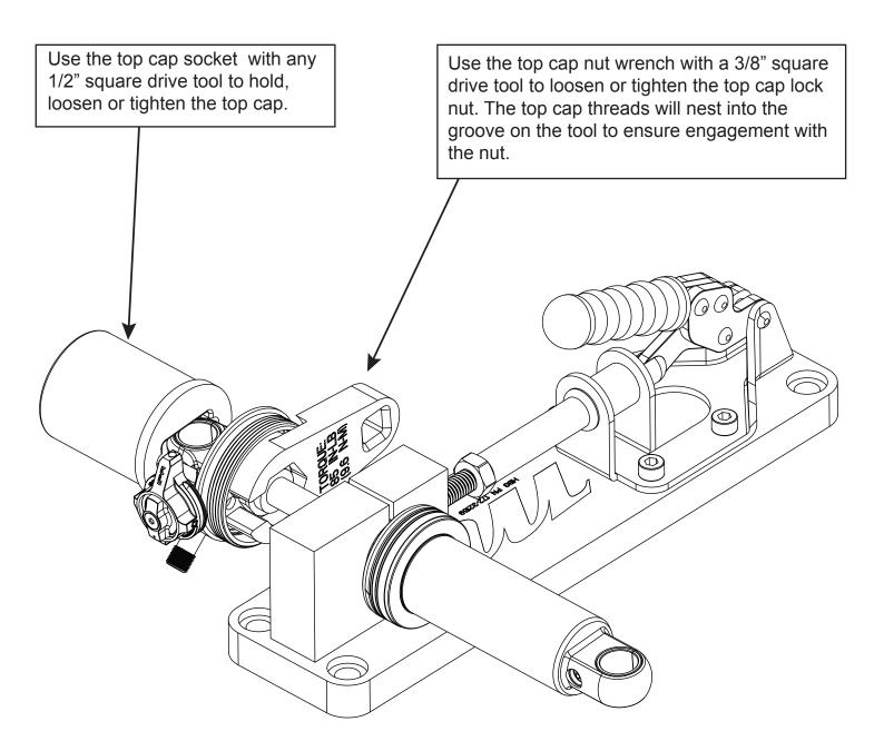
Use the clamp block to hold the shock shaft for service. Part number for the clamp block is 172-32159-K001.
