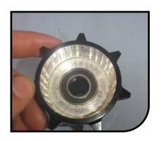
Lightly grease and press in the drive side (DS) bearing on the freehub body.
