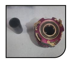
Install the spacer, lightly grease and press in the none drive side (NDS) bearing.
