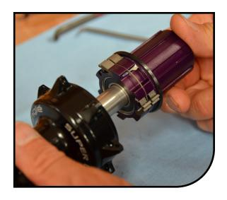
Once the freehub body is resting on the hub, depress all three pawls of the first set and push down, this will allow the freehub to move into the hub up to the second set of pawls. If the freehub body is difficult to install, gently rotate counter clockwise as it is pushed into the hub shell. Repeat for the second set of pawls. Note: Bubba X and Super Bubba X have one row of 6 pawls
