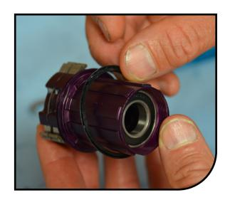
Lubricate with pawls and springs with free hub Body grease for quieter operation and longer service life, use free hub oil for louder operation and improved low temperature operation.
