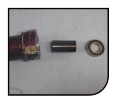
Pull out the outer bearing on the freehub body.
