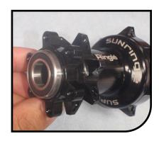
Pull out the drive side bearing.
