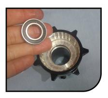
Pull out the inner bearing on the freehub body, behind this bearing is a spacer.
