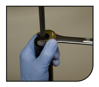
Remove Compression Rod Assembly from the inner leg.
