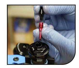
Attach the empty syringe with Dorado Cartridge bleed fitting to top-cap bleed port.
