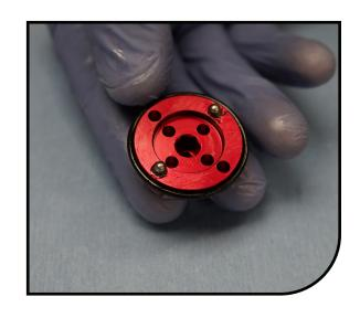
Install the TPC+ adjuster knob onto the end cap and secure with the 2mm screw.
