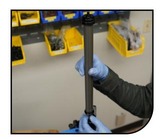
Install the high speed adjuster onto the end cap. Be sure that O-ring # 100-025 below the adjuster is in place and greased. Secure the adjuster with the c-clip (Retaining ring pliers can be used to aid in the installation).
