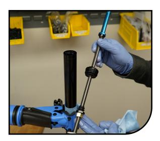
Carefully remove the A) glide ring (129-27922-L013), B) back up ring (129-31523-L338) and C) air piston quad seal (110-215). We recomend using a plastic pick to ensure the piston is not damage.
