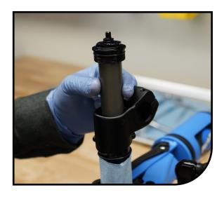
Replace the following O-rings on the rebound damper assembly.
