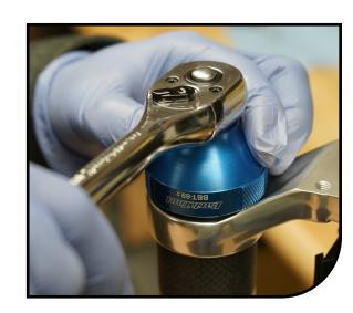
Loosen the pinch bolts on the lower crown and remove the damping leg from the fork. You will need to remove the frame bumpers to do so. Put them in a safe place so you do not misplace them.
