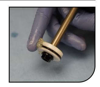
Use a cassette tool to tighten the IRT end cap to a proper torque of 6.8 - 9.0 Nm [60-80 in lb].
