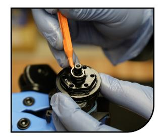
Adjust HSC to min, then turn LSC asjuster counter clockwise to remove the LSC adjuster from top-cap. Place damper top-cap over catch pan. Cycle damper shaft several times to cycle out old oil from damper.
