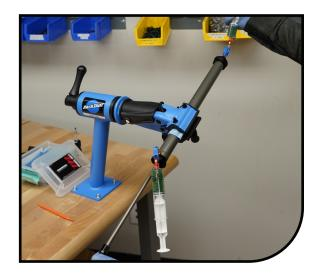
Closing the bleed hose clamp on both syringes cycle the damper SLOWLY to draw air to the top of the damper. Open bleed hose clamps and repeat step 3 and 4 until no air bubbles are present in oil drawn into upper syringe.
