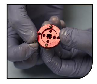
Place O-ring # 100-024 around the TPC+ knob and apply a small amount of grease to it.
