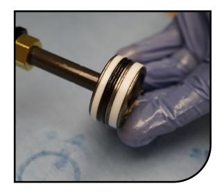
Wrap the inner leg in a towel and gently clamp in a bike stand with the drop out pointing up. While holding the drop out remove the IRT assembly using a casstte tool.
