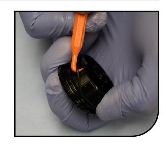
Install the top cap onto the end of the compression rod. Use a 16 notch Bottom Bracket Tool and a 13mm wrench to tighten to the proper torque of 3.4-4.5 N m (30-40 in lb)
