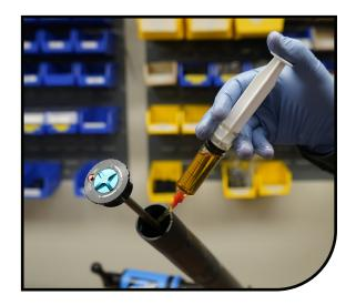
Fully extend the inner leg and 15 tighten down the top cap using a 16 notch Bottom Bracket Tool to the proper torque of 6.8-9.0 N m (60-80 in lb). Reinstall the damping leg into the fork crowns on the bike.
