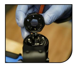
With the forks steerer tube clamped in a bike stand oriented upright. Loosen the upper clamp while leaving the lower tight. (This will allow the top cap to be loosed without the leg spinning.) Loosen the damping leg top cap using a 16 notch Bottom Bracket Tool. Only loosen the top cap at this point. Do not remove it.
