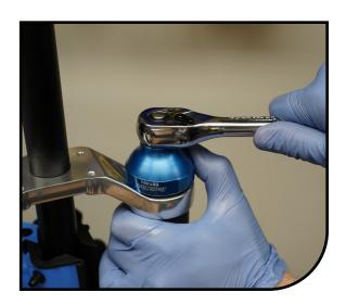
Loosen the pinch bolts on the lower crown, and remove the leg from the fork. Be sure not to misplace the frame bumper that will need to come off the fork leg.
