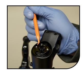
Install the assembly in the inner 3 leg by sliding it into the bottom of the leg.
