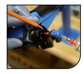
Simultaneously compress the filled syringe and retract the empty syringe to remove air from the damper. Refill the syringe as needed until oil is drawn into the damper upper syringe.
