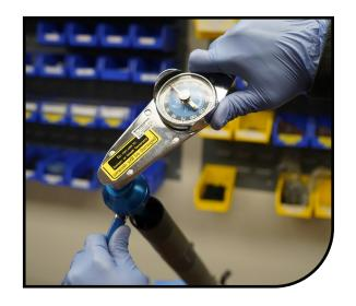
Fully extend the inner leg and tighten down the top cap to the proper torque of 6.8-9.0 N m (60-80 in lb). Fill the fork to the desired air pressure.
