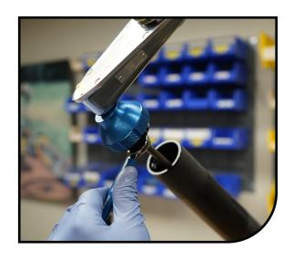
Install the rebound knob into the top cap by snapping it into place. Fully close the rebound by turning the knob clockwise. Fully extend the rebound shaft, pulling the inner leg up into the outer leg.
