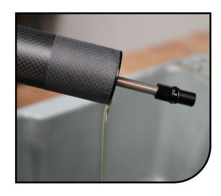
Wrap the inner in a rag and clamp it lightly in the bike stand with the compression rod pointing towards the ceiling.
