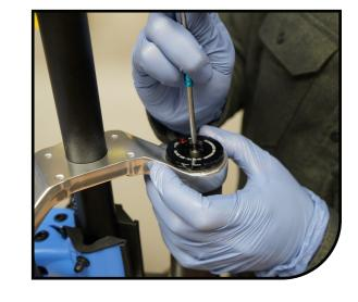
The air spring leg top cap needs to be loosened. Loosen the pinch bolt on the top crown, and crack the top cap loose with a 16 notch Bottom Bracket Tool.
