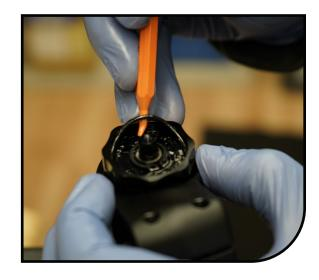
Next you will remove the High Speed adjuster knob. Remove the c-clip that holds the knob on using a snap ring pliers or similar tool.
