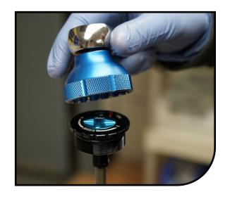
You will now remove the top cap from the rebound shaft. Place a 12mm wrench on the flats of the rebound shaft and use a 16 notch Bottom Bracket Tool to unthread the top cap from the shaft. Once the top cap is unthreaded, remove the rebound knob from the top cap.
