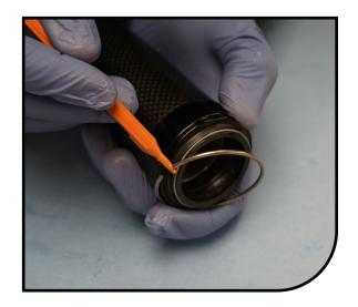
Gently pry out the old dust seal from the outer leg. A tool we have found that works well is a downhill tire lever. If using a flat blade screwdriver to remove the seal be careful the tip of the blade does not catch on the lip inside the outer leg.
