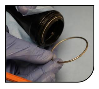
Gently pry out the old dust seal from the outer leg. A tool we have found that works well is a downhill tire lever. If using a flat blade screwdriver to remove the seal be careful the tip of the blade does not catch on the lip inside the outer leg.
