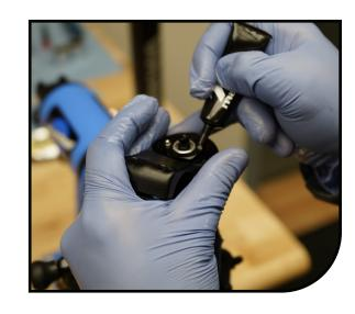
Install the ABS+ adjuster knob onto the end cap and secure with the 2mm screw.
