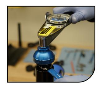
Install top cap into the outerleg. Using a 16 notch bottom bracket tool tigthen to 6.8-9Nm {60-80 In-Lb}.
