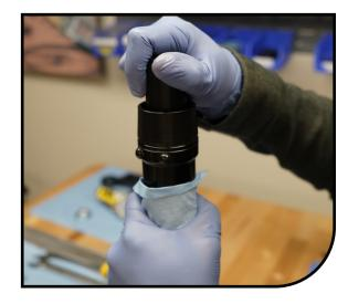
Install the wear ring back onto the outer leg.
