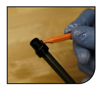
**B.** O-ring # 100-026 - This is the O-ring that is around the outside of the compression assembly top cap.
