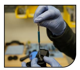
Using a 20mm socket loosen the bottom spring cap. Then gently remove the cap and spring by pulling them out of the leg.
