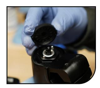
First step is to loosen the damping leg top cap using a 16 notch Bottom Bracket Tool. It helps if the leg is still clamped in the lower crown assembly while breaking the top cap loose (be sure the upper crown is loosened, you only want the lower tightened when breaking loose the top cap). Only loosen the top cap at this point. Do not remove it.
