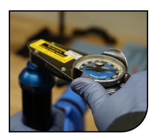
Using the sag guide tool to spread the crowns, slide the leg into the crown, align to proper wheel size and tighten crown bolts to 10.7-12.4 Nm {95-110 In-Lb}.
