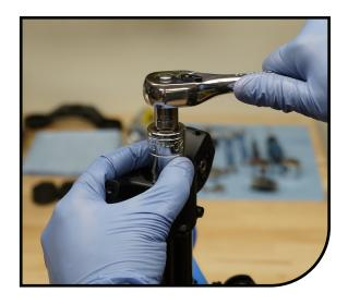
Loosen the pinch bolt on the top crown, and crack the top cap loose with a 16 notch Bottom Bracket Tool.
