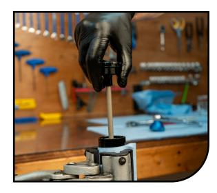
13 After you have properly set the oil height fully extend the inner leg and tighten down the top cap using a 16 notch Bottom Bracket Tool to the proper torque of 6.8-9.0 N m (60-80 in lb).
