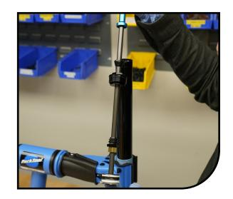
Carefully remove the glide ring (129-27922-L013), back up ring (129-31523-L338) and air piston quad seal (110-215). We recomend using a plastic pick to ensure the piston is not damage.
