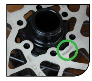
Using a T25 Torx driver, install, tighten, and torque the disc screws to 50±5 in lbs  $(5.65\pm0.56 \text{ N m})$ , in a star pattern sequence.
