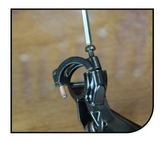
\*Optional, install either Shimano™ or SRAM™ PeaceMaker clamp. Torque bolts to  $30\pm5$  in lbs  $(3.39\pm0.56 \text{ N m})$ .
