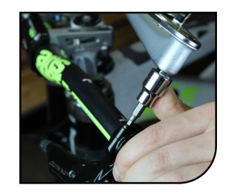
Adjust pad contact by turning adjuster screw in the "+" direction to add stroke or in the "-" direction to reduce stroke.
