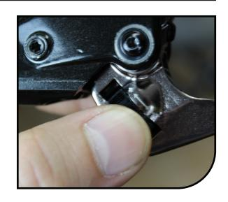
To adjust the tool free lever T2 reach on the T2, turn the 2mm hex screw with a 2mm hex wrench located on the front of the lever. Turning it in the counterclockwise direction will move the lever in. Turning it in the clowise direction will move the lever out. Do not force the screw beyond its limits.
