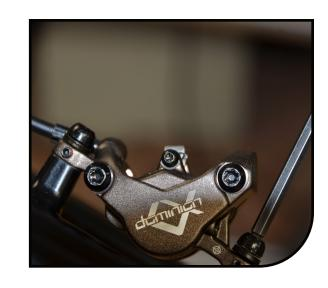
Squeeze the lever blade a minimum of 5 times to seat the caliper pistons.
