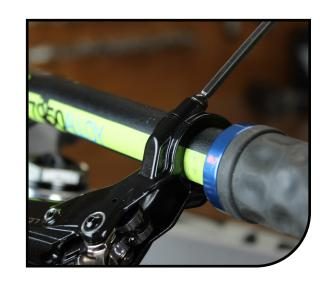
Once you have set the master cylinder in the final desired position on your handlebars, tighten down the top mount bolt. Torque to 30±5 in lbs  $(3.39\pm0.56 \text{ N m})$ . Next tighten down the other bolt to a torque of  $30\pm5$  in-lb  $(3.39\pm0.56$  N m).
