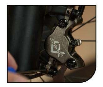
Torque the lower mount bolt (A) to  $80\pm5$  in lbs  $(9.0\pm0.5 \text{ N m})$ . (the upper adjuster screw keeps the caliper from rotating out of alignment). Torque the upper mount bolt (B) to 80±5 in lbs  $(9.0\pm0.5 \text{ N m}).$
