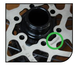
Using a T25 Torx driver, install, tighten, and torque the disc screws to 50±5 in lbs  $(5.65\pm0.56 \text{ N m})$ , in a star pattern sequence.
