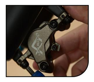
Using the 2mm hex tool, turn the adjuster screws clockwise until they contact the mount bolts.
