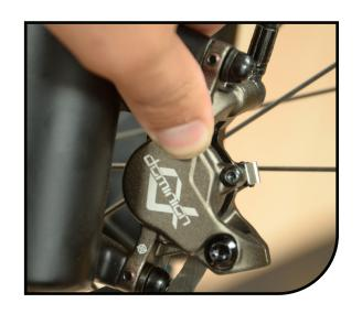
Snug the mount bolts using the 5mm hex tool while keeping the outer pad against the disc.
